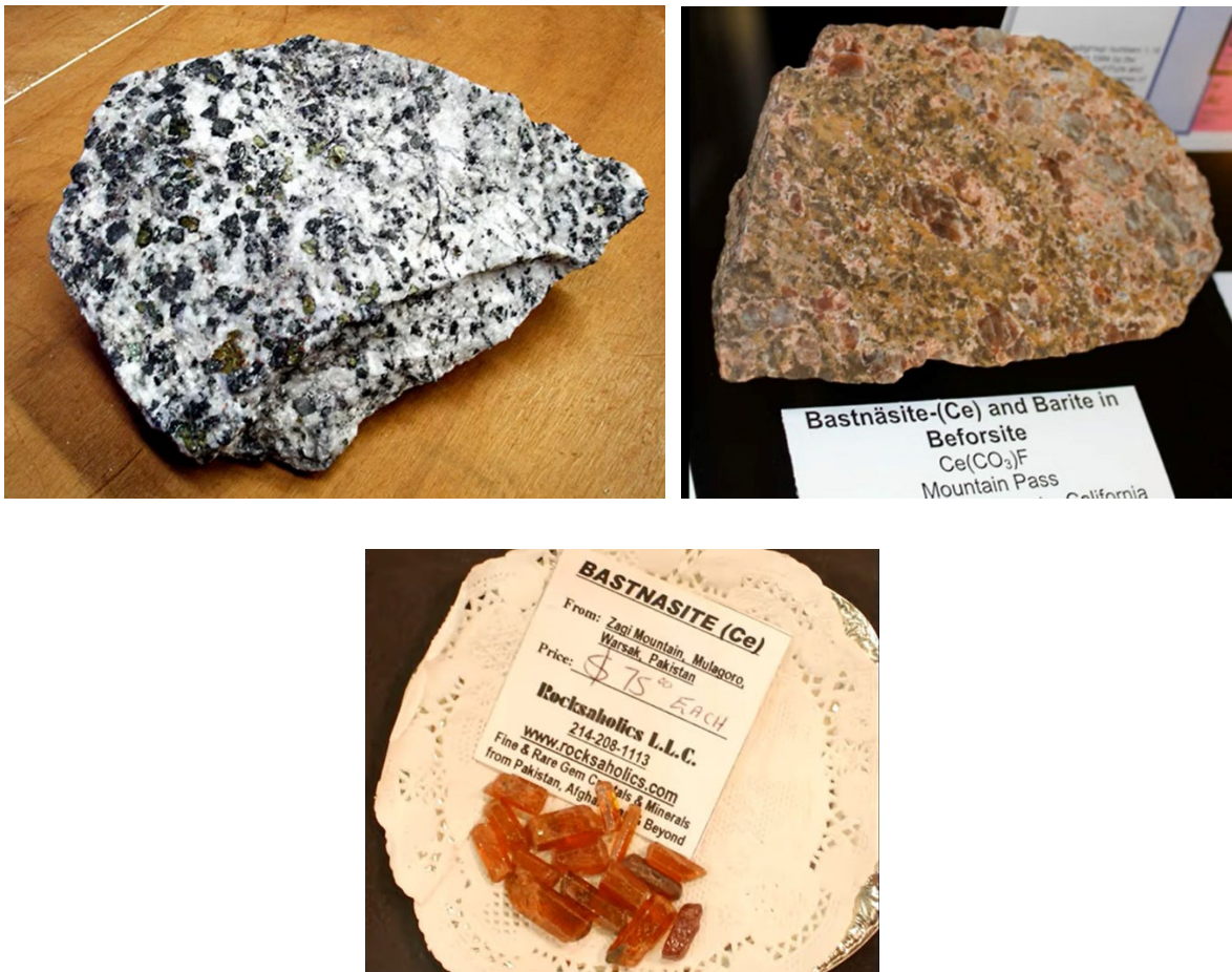
Figure 14. Carbonatite ore, Bastnasite ore Ce(CO_3)F Mountain Pass, California, Bastnaesite crystals, Zagi Mountain, Pakistan [11].
