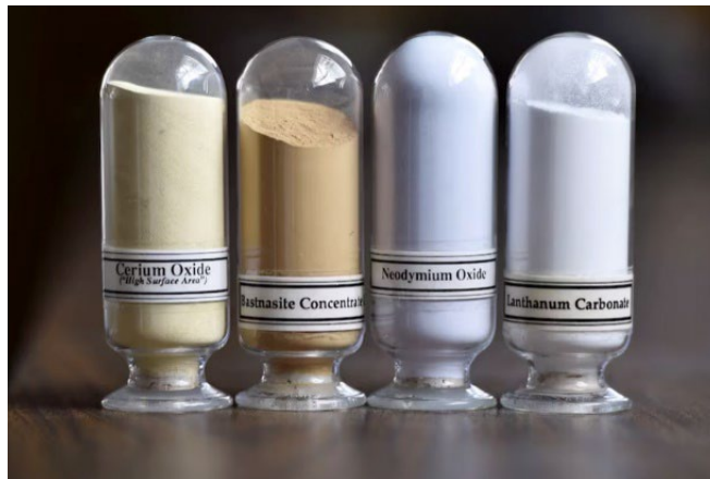
Figure 9. Rare Earths compounds samples. Cerium oxide, Bastnaesite ore concentrate, Neodymium oxide, Lanthanum carbonate. Source: Molycorp corporation.
