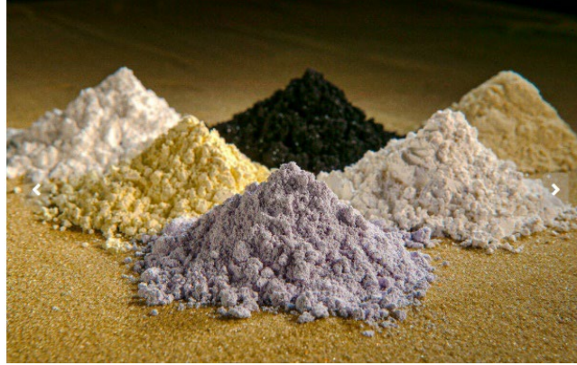
Figure 8. Rare Earths Elements concentrates. Clockwise from top center: Praseodymium Pr, Cerium Ce, Lanthanum La, Neodymium Nd, Samarium Sm and, Gadolinium Ga [2].
