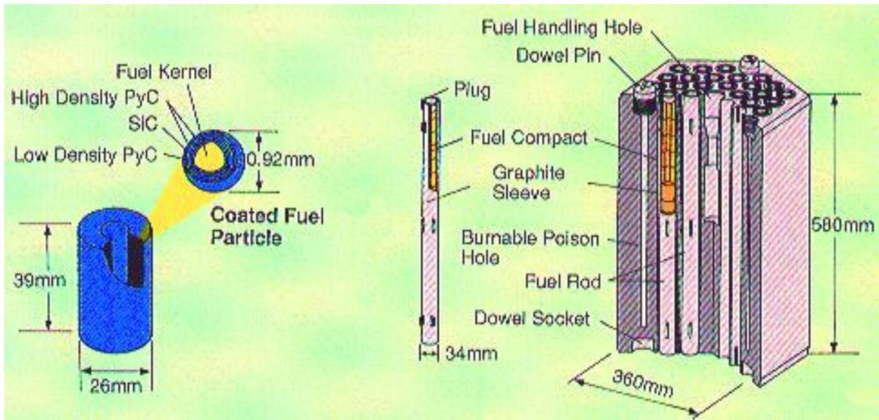
Figure 6. Prismatic graphite fuel assembly in the HTTR.
