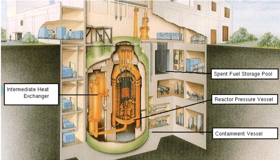
Figure 5. High Temperature Gas Cooler Reactor, HTTR, Japan.
