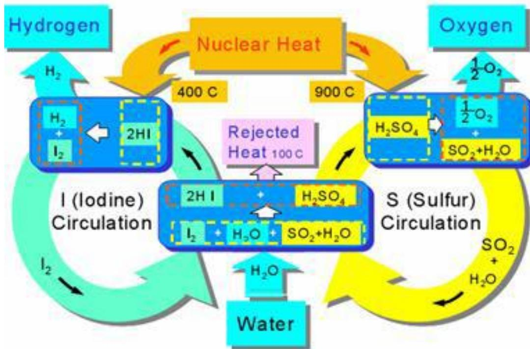
Figure 1. Sulfur Iodine process for hydrogen production operates at 900 degrees C.
