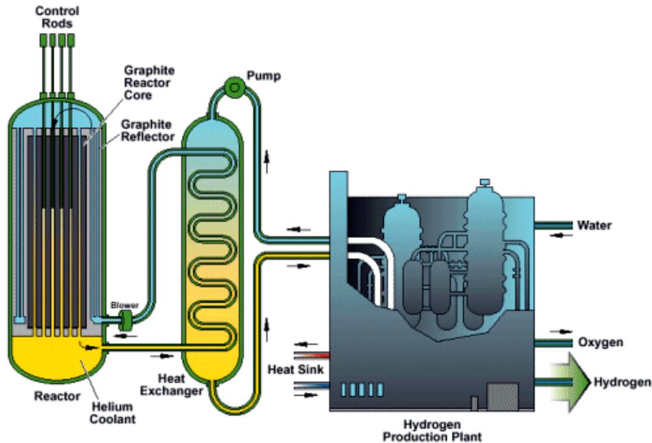
Figure 2. Very High Temperature Hydrogen and Electricity (VHTR) design.
