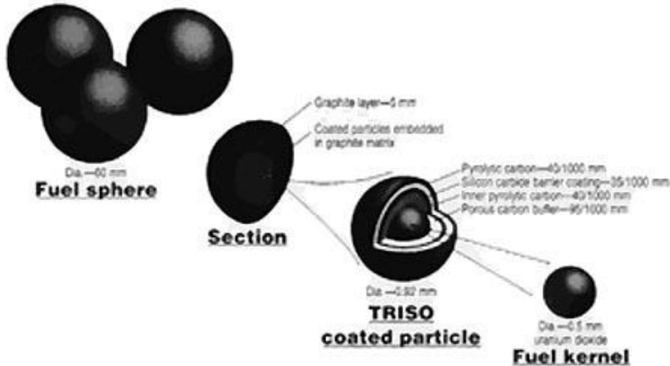
Figure 3. Fuel elements used in the Pebble Bed Modular Reactor (PBMR).
