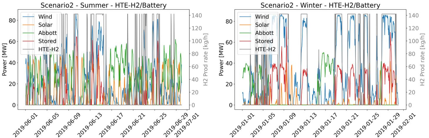
Figure 10. Scenario 2 hourly electricity distribution by source for an increase capacity factor of 10. The storage mechanisms are HTE-H2 and Li-ion batteries.
