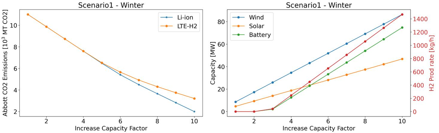
Figure 9. CO<sub>2</sub> emissions, wind, solar, and storage capacities for different increase capacity factors in the winter month.
