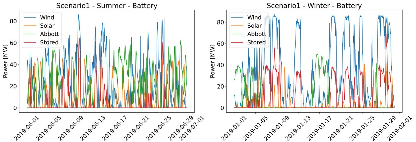
Figure 7. Scenario 1 hourly electricity distribution by source for an increase capacity factor of 10.
