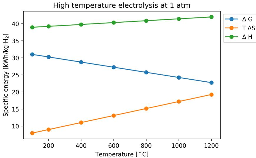
Figure 3. Energy required by electrolysis at atmospheric pressure [1].
