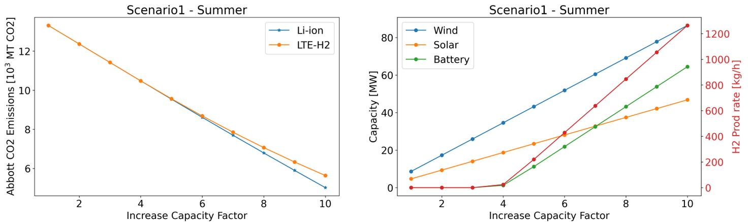
Figure 8. CO<sub>2</sub> emissions, wind, solar, and storage capacities for different increase capacity factors in the summer month.
