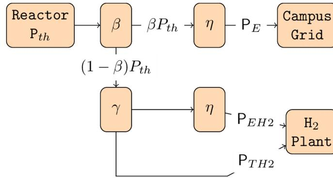
Figure 5. Diagram of a nuclear reactor coupled to a hydrogen plant [1].
