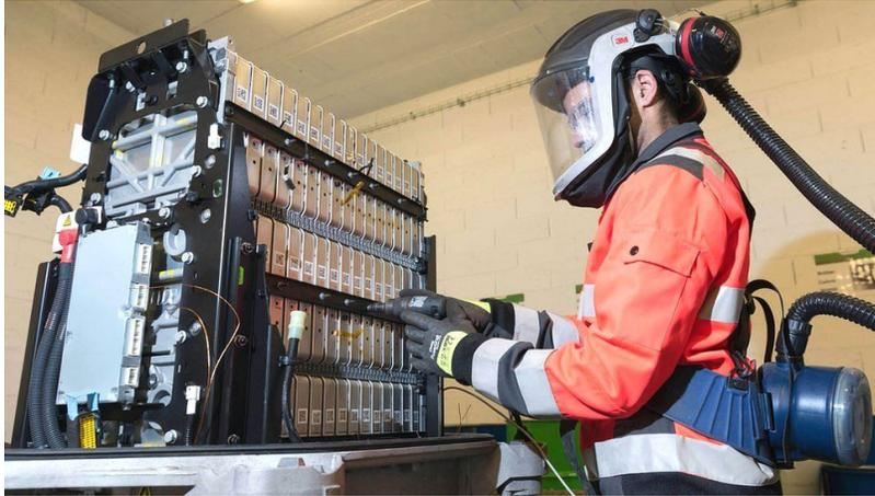
Figure 2. Safety features used in the dismantling a Renault electrical vehicle battery.
