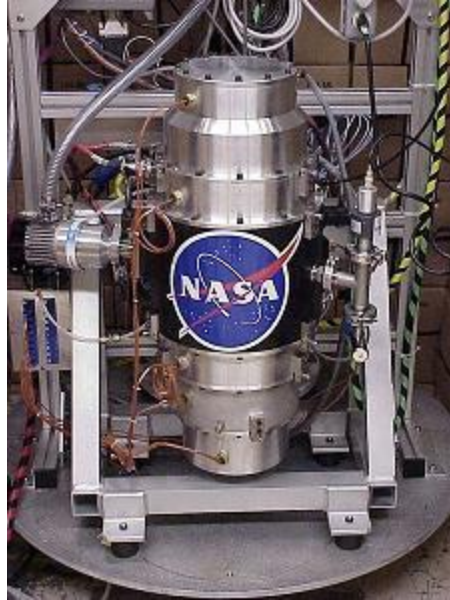
Figure 2. G2 flywheel with a rotational speed of 41,000 rpm. Source NASA.
