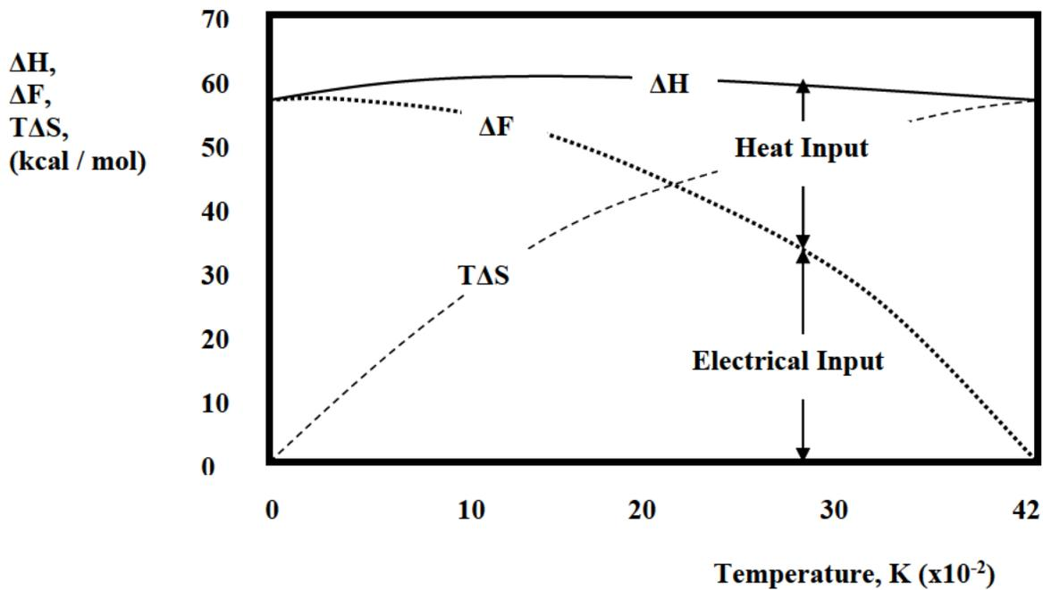
Figure 1. Energy splits for water decomposition as a function of temperature in the High Temperature Electrolysis (HTE) process [1].
