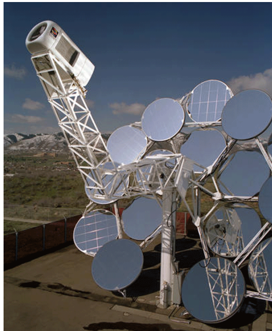
Figure 39. Stirling Engine multiple dishes solar energy collector. Source SAIC.
