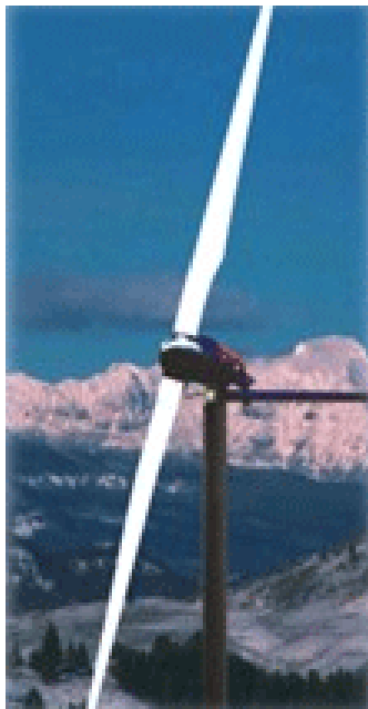
Figure 3. Whisper 500, 3 kW wind turbine.
