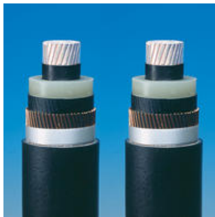
Figure 34. HVDC Light cables pair, 43 mm, 2 kg/m Al conductor 340 mm 2 . Source: ABB.
