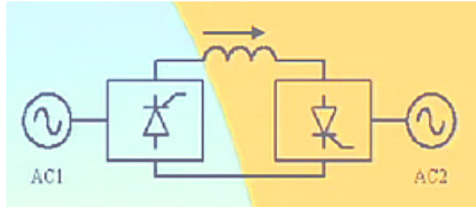
Figure 21. Conventional HVDC with Current Source Converters (CSCs) uses Thyristor valves. Source: IEEE.
