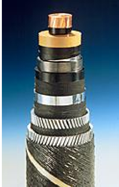
Figure 29. Layers of a submarine electrical power transmission cable. These cables are mass impregnated (MI) cables suitable for HVDC. The cable has a copper conductor and the insulation is made of oil impregnated paper. There is a lead alloy sheath outside the insulation. Mechanical protection is achieved by steel tape and steel wire armoring. A typical 450 kV HVDC cable has an outer diameter of approx. 13 cm. Source: ABB.
