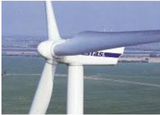
Figure 5. The Vestas V90 3MW rated power wind turbine is an example of the economy of scale characteristic of utility scale large wind turbines. Source: Vestas.
