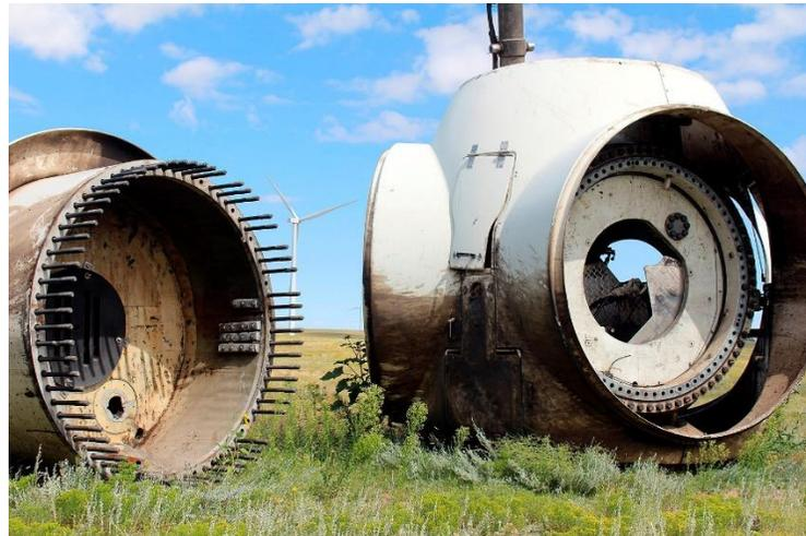
Figure 3. Hubs awaiting recycling.
