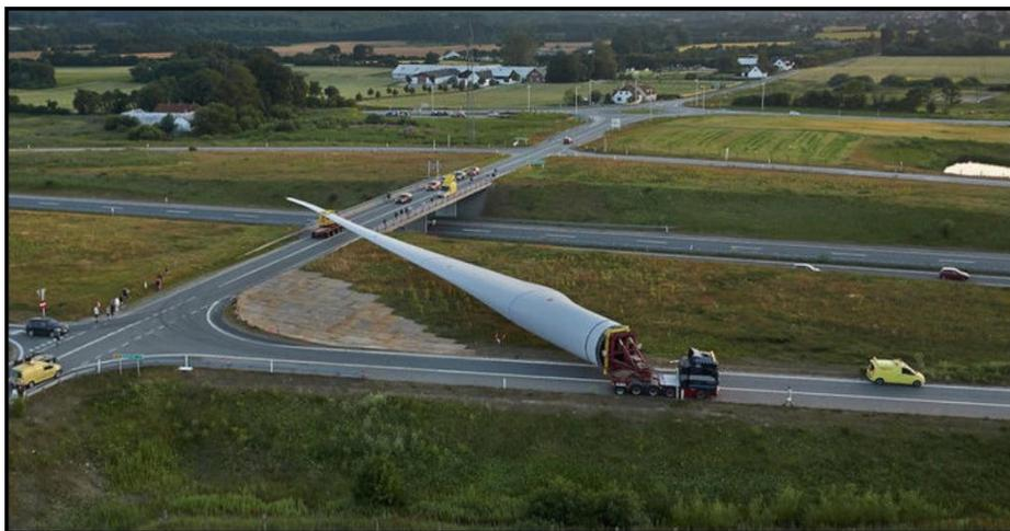
Figure 5. Transportation difficulty of large size rotor blades at roads intersections, bridges and overpasses.
