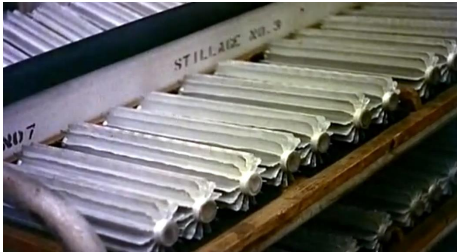
Figure 8. Aluminum-clad uranium fuel elements used in the Windscale reactors. Notice the manufacturing nicks defects in the Aluminum fins which may have caused the frequent fuel channels obstructions.
