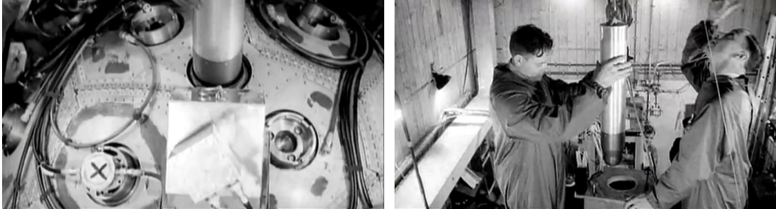
Figure 17. First UK plutonium implosion device pit being inserted into the explosive lenses assembly.
