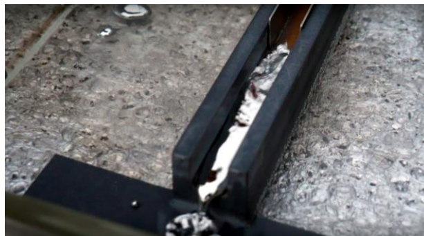
Figure 13. Liquid metal MHD pump. Perpendicular electric and magnetic fields generate the force moving the liquid metal which is a eutectic liquid metal alloy at room temperature composed of of Pb, Bi, tin and indium.
