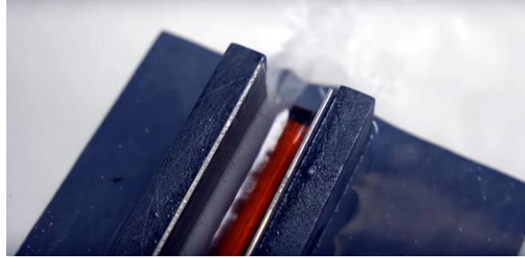
Figure 12. Ionized water propelled by a MHD pump. It may silently propel a naval vessel silently without moving parts as in the “caterpillar drive” in the movie: “The Hunt for Red October.” An impediment is the generation of bubbles of hydrogen caused by the electrolysis of the water.
