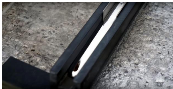
Figure 12. Ionized water propelled by a MHD pump. It may silently propel a naval vessel silently without moving parts as in the “caterpillar drive” in the movie: “The Hunt for Red October.” An impediment is the generation of bubbles of hydrogen caused by the electrolysis of the water.
