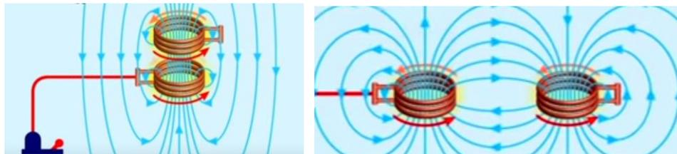
Figure 7. Principle of magnetic induction and highly coupled magnetic resonance for harvesting electromagnetic energy.
