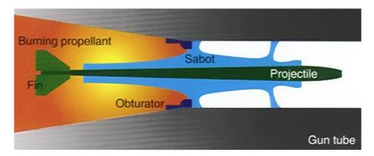
Figure 9. Cross Section of sabot showing kinetic energy transfer from the propellant to the sabot.
