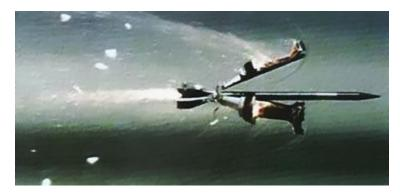
Figure 8. The sabot detaching from a depleted uranium projectile.
