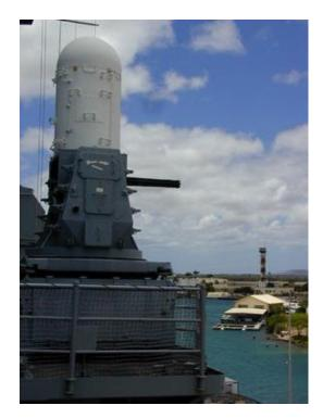
Figure 3. Depleted Uranium Gatling gun radar assembly on the USS Missouri, Pearl Harbor, Hawaii, for interception of oncoming missiles and attacking fast boats. Photo: M. Ragheb.
