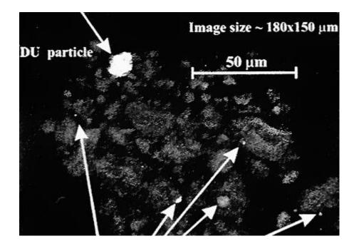
Figure 15. Depleted uranium particles can be detected in contaminated soil using a Scanning Electron Microscope (SEM) that is equipped with an Energy Dispersive X-ray Fluorescence detector.
