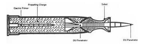
Figure 7. Schematics of a sabot armor piercing rounds with a depleted uranium penetrator.
