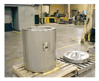
Figure 12. Depleted Uranium used as a DUCRETE concrete aggregate in a radiation shielding cask.
