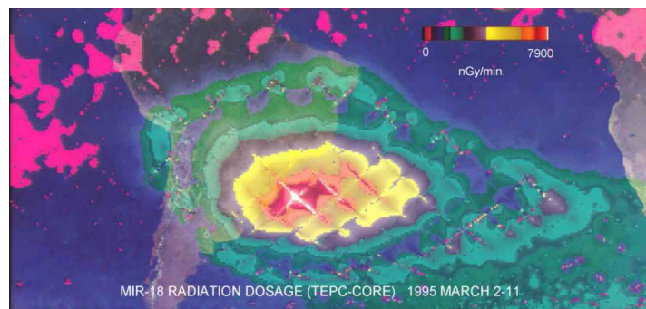
Figure 19. Dose rate to the MIR-18 Space Station showing the South Atlantic Anomaly just east of the Brazilian coastline.
