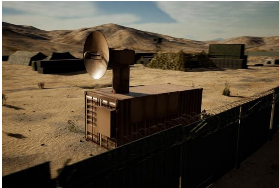
Figure 4. USA Air Force Research Laboratory's Tactical High-power Operational Responder, or THOR. THOR is a portable counter Unmanned Aircraft Systems-UAS system, capable of destroying swarms of drones at speed-of-light, at long range, in its base defense mission. Source: Air Force Research Laboratory.
