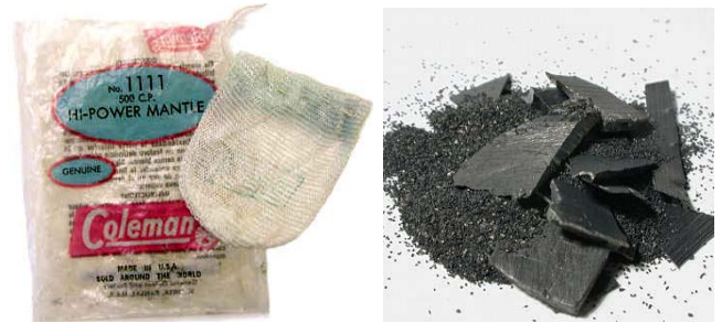
Figure 2. Thorium dioxide with 1 percent cerium oxide impregnated fabric, Welsbach incandescent gas mantles (left) and ThO 2 flakes (right). Yttrium compounds now substitute for Th in mantles.
