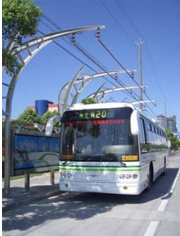
Figure 8. Bus running on ultra capacitors charges up at a bus stop every 3-5 miles for fast recharging. Photo: Sinautec Automobile Technologies.
