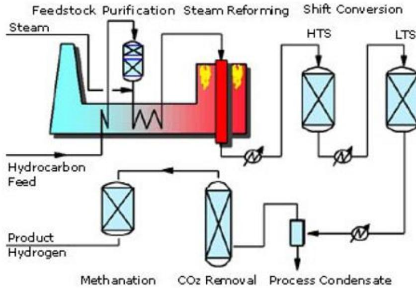
Figure 2. Steam reforming for hydrogen production.
