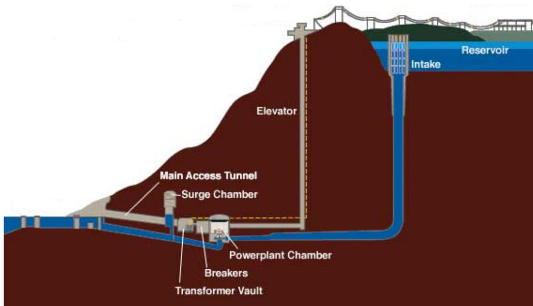
Figure 1. Pumped Storage system configuration.
