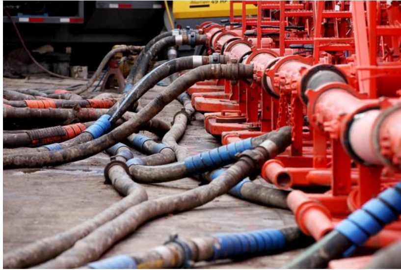
Figure 16. Mixing water and sand at a 6,600 psi pressure. Marcellus formation, Camptown, Pennsylvania. Hydraulic fracturing is being used to pump natural gas out of about 3,000 wells in the USA, with 120 to 150 wells being added every month. The actual procedure lasts only about a week, and then the operating team moves on to the next on a long list of wells. Source: Southwestern Energy Co.
