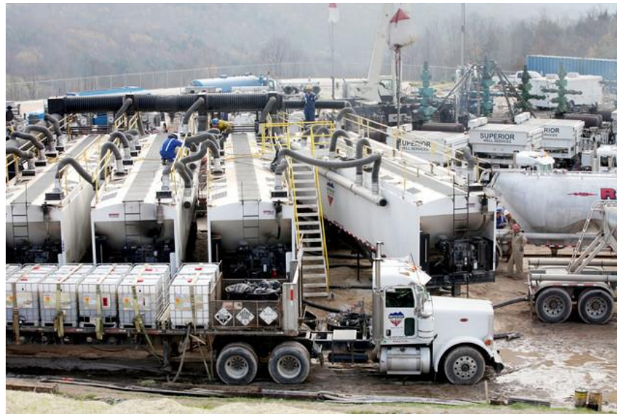
Figure 18. Sand and water mixing at the Marcellus formation, Camptown, Pennsylvania. Trucks bring giant 2,400 horsepower pumps to the site, where about a dozen of these are connected. A fluid and sand mixture at about 1,000 bar is forced into the deposit. The mixture consists of millions of liters of water, special sand and chemicals designed to kill bacteria that could inhibit the flow of gas. Source: Bloomberg.
