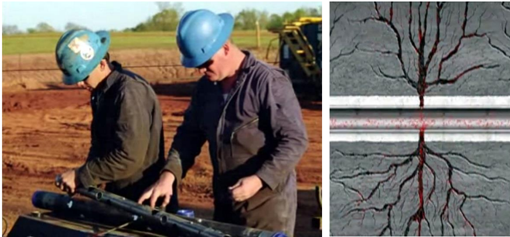
Figure 14. Fracturing gun and generated fractures around horizontal well bore.
