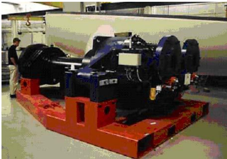
Figure 16. Wind generators gear boxes increase the rotational speed and decrease the torque rather than the opposite in other industrial equipment. A 600-750 kW wind turbine uses a gear ratio of 1 to 50.
