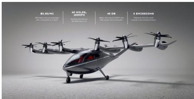
Figure 3. Technical Specifications of electric eVTOL aircraft. The operational cost is expected to be \$3.30 per mile travelled. It has a 60 mile range, can fly at 150 mph and can carry 4 passengers with 1 pilot. The plane will have a take-off weight of less than 7,000 pounds.
