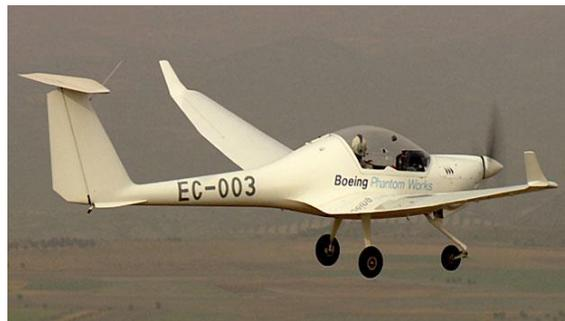
Figure 4. Hydrogen Fuel cell Aircraft designed by the Boeing Company Research And Technology (BRAT) division; formerly Phantom Works was first flown in Spain.
