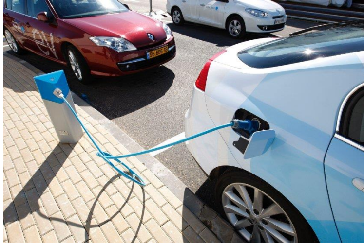
Figure 2. Electrical car battery recharging station.
