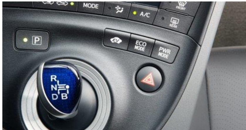
Figure 6. Toyota Prius Hybrid Electric Vehicle, HEV power controls.
