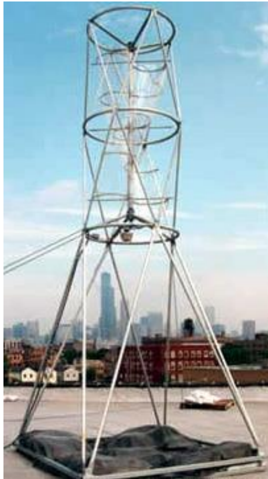
Figure 15. Vertical 510V turbine with ballast.
