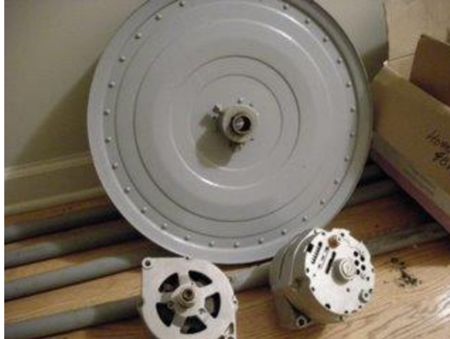
Figure 18. Ribbed helical rotors construction, transmission base and alternator detail of helical vertical turbine.
