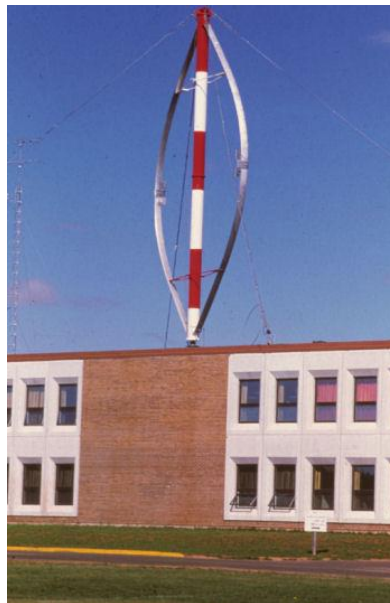
Figure 3. An Indal Darrieus vertical axis turbine built on a school roof in eastern Canada around 1980. The turbine was reported to be removed because of the damage it caused to the building. Source: NR Canada.
