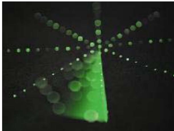
**Fig. 1: Radar screen interference pattern from wind turbines.**
