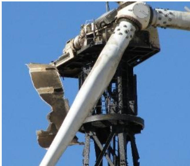
Figure 3. Decaying abandoned truss tower style wind turbine in California.
