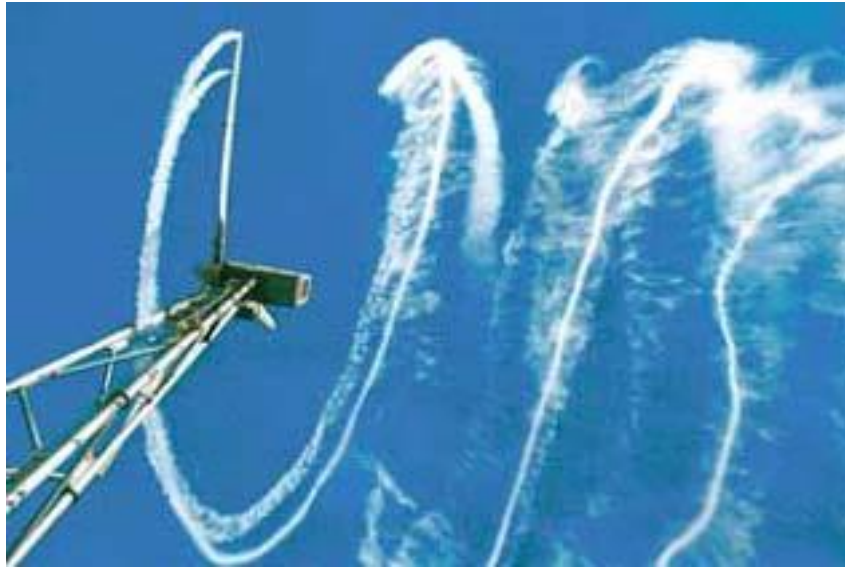
Figure 4. Wake effect from wind turbine shown with smoke generated at a single blade turbine rotor's tip. This turbine rotates clockwise, whereas most turbines rotate counterclockwise. Source: Risø National Laboratory, Denmark.
