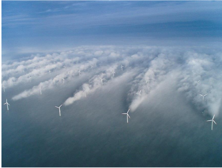
Figure 7. Wake from offshore wind turbines at Horns rev west of Denmark. Photo: Vattenfall.
