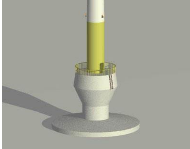
Figure 15. Gravity support foundation for offshore wind turbine.
