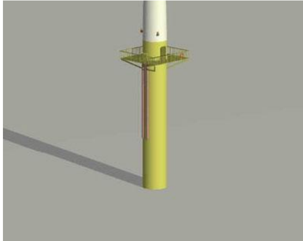
Figure 13. Monopile support for offshore wind turbine.
