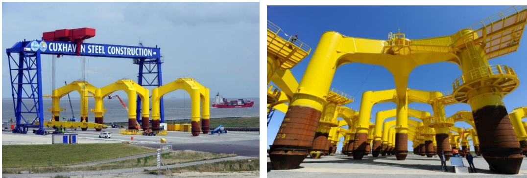
Figure 16. Foundations welding for North Sea wind farms installations, Germany. Source: DPA.
