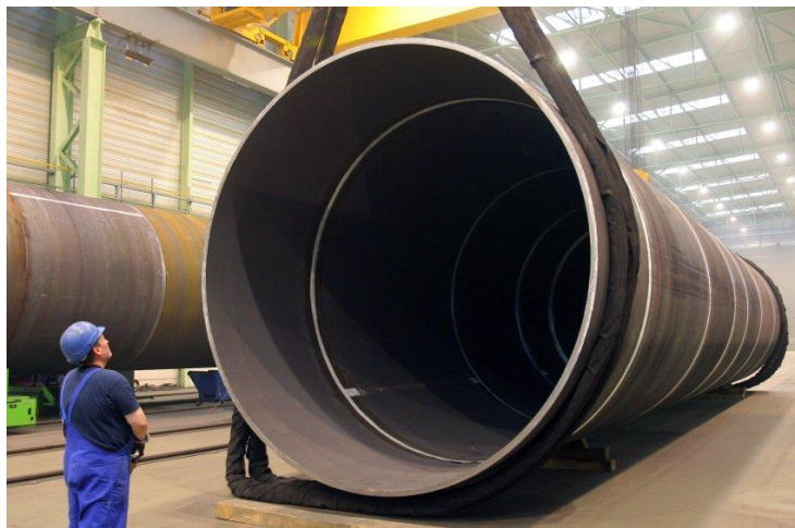
Figure 12. Steel tower manufacture for offshore wind turbine in the Baltic Sea.
