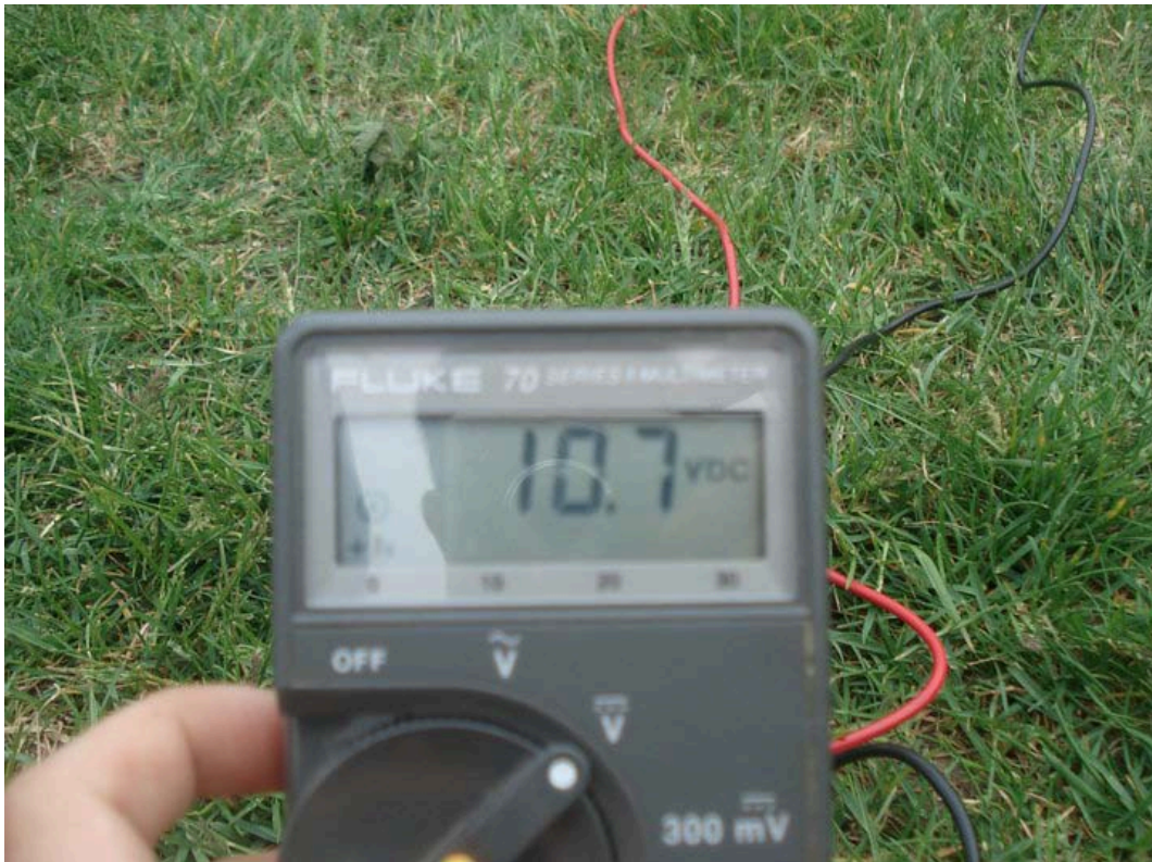
Fig. 6: Multimeter used for generator output voltage readings.
