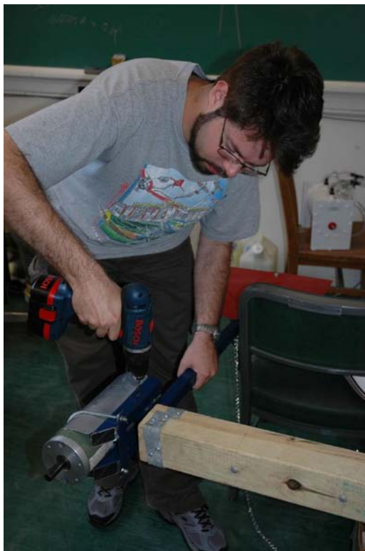
Fig. 3: Drilling of nacelle mounting bolt holes in frame.
