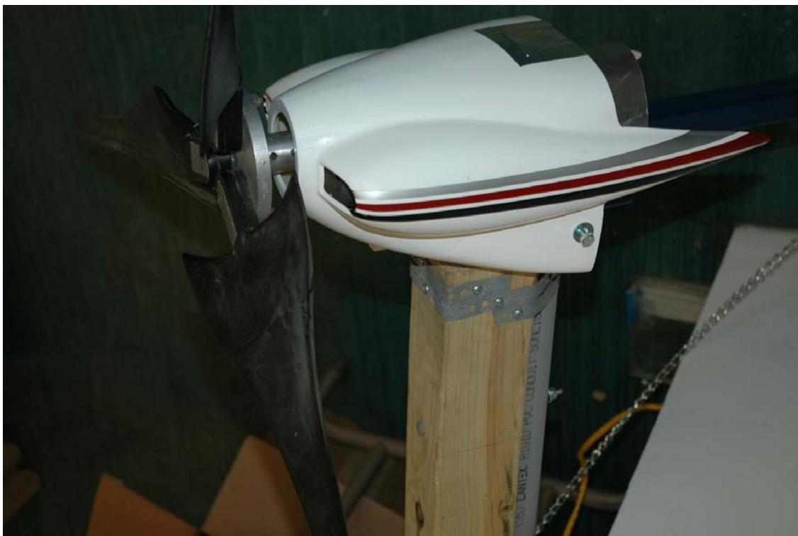
Fig. 4: Finished nacelle installation.
