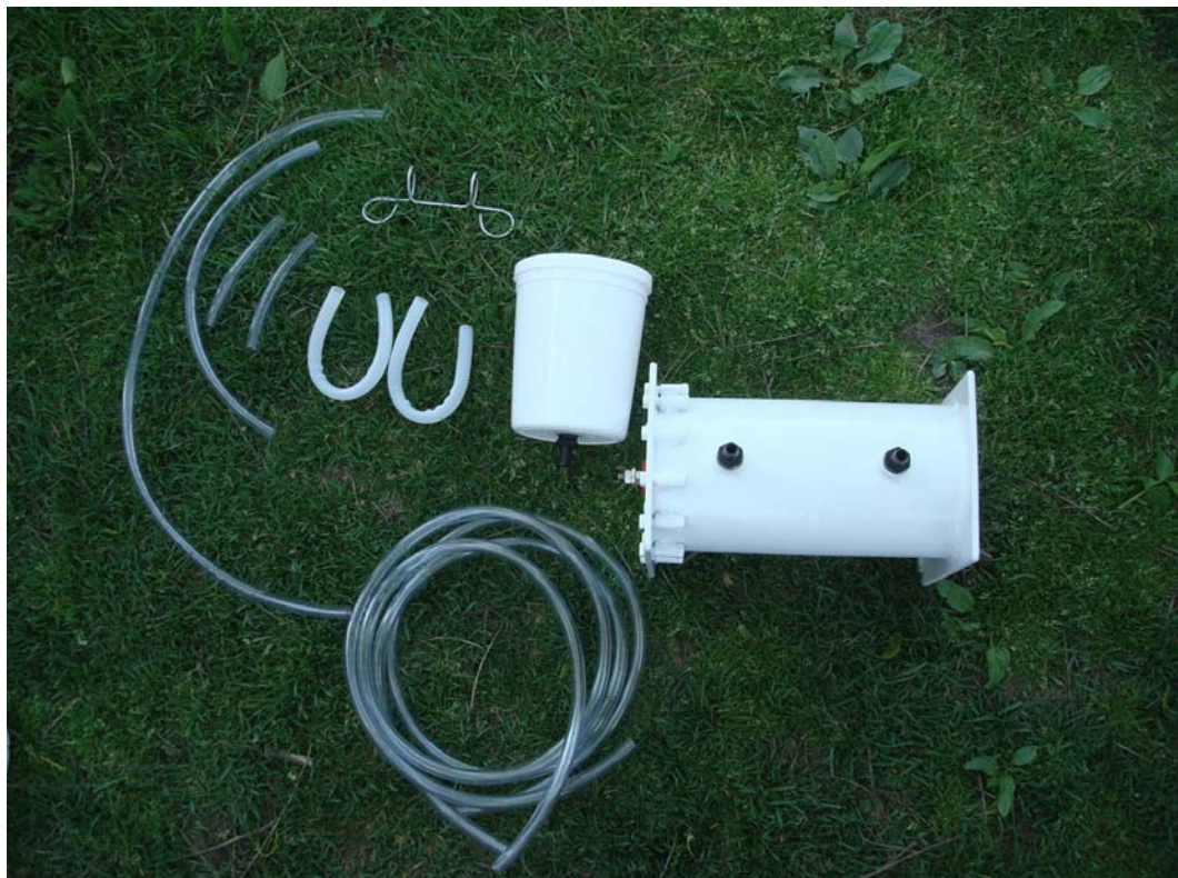
Fig. 7: Electrolyzer system prior to assembly.
