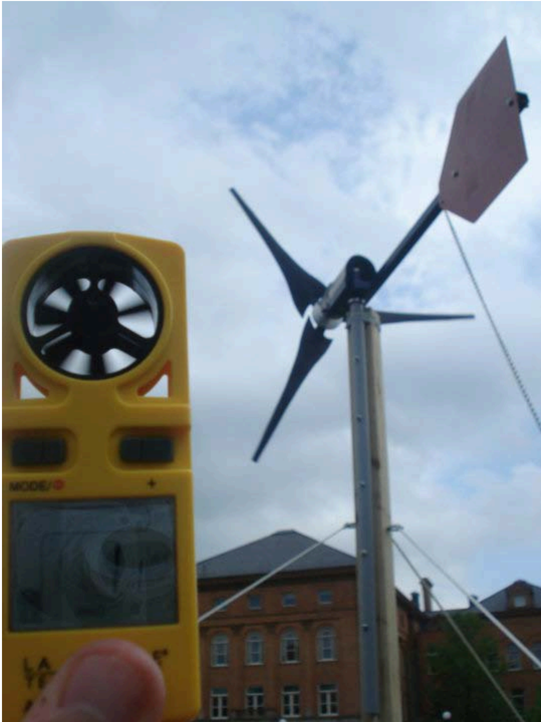
Fig. 5: Installed turbine and anemometer for wind speed vs. generator voltage measurements (I'm holding the "yaw mechanism" chain).
