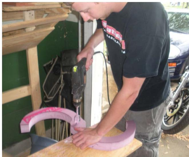
The centers were then bored at 1 3/8" to fit over the pipe we bought. The 1" pipe meant it had an inside diameter of 1", while the outside was a nominal 1.315 inches, which presented a problem further down the line.
