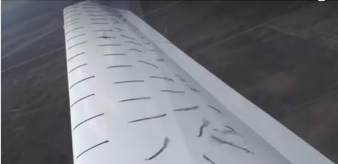
Figure 6. Flow separation and loss of lift at a steep angle of attack.
