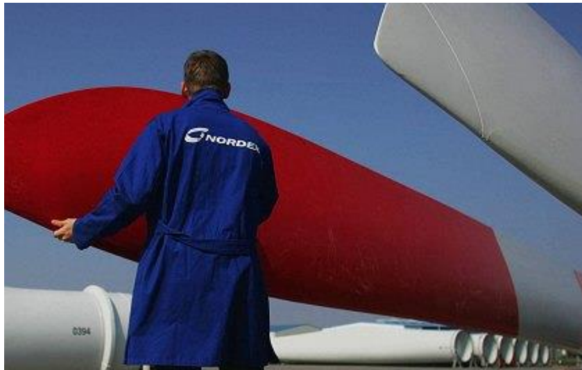
Figure 1. Inspection of rotor blade tips for possible cracks. They are subjected to wind speeds reaching 250 km/hr. Source: Nordex.
