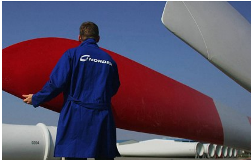
Fig. 1: Inspection of rotor blade tips for possible cracks. They are subjected to wind speeds reaching 250 km/hr. Source: Nordex.
