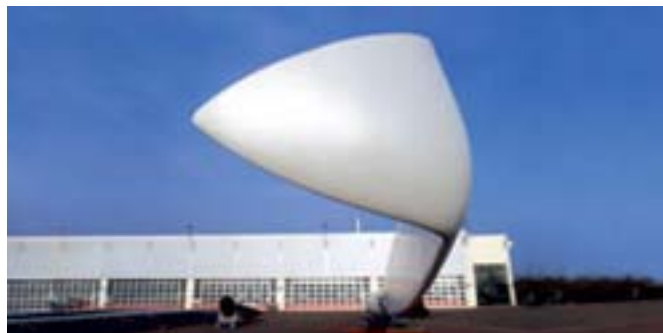
Figure 9. Winglets at rotor tips to reduce the noise effect. Source: Enercon.
