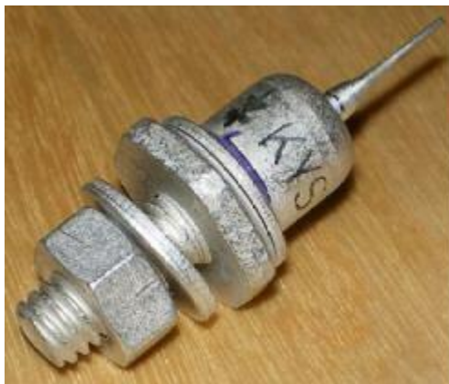
Figure 8. Schottky diode rated at 30 Amps and maximum voltage rating of 40 volts.
