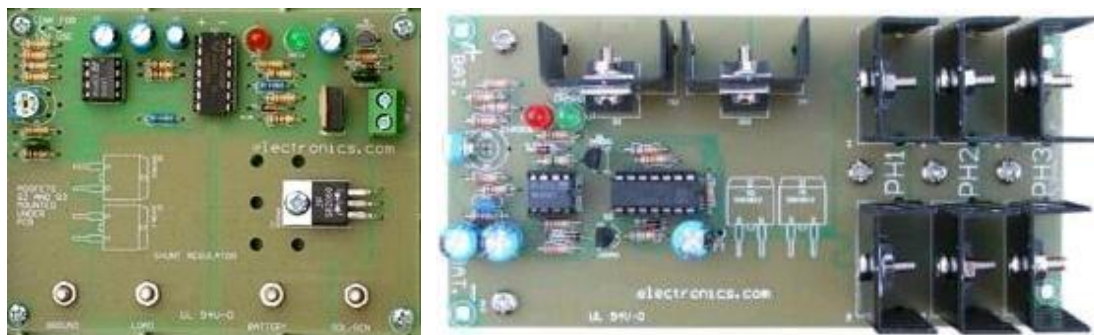
Figure 13. DC on the left, and three phase with a built in three phase bridge rectifier, on the right, AC charge controllers. The regulators are rated at a current handling capacity of 20 Amps AC and 23 Amps DC. They can be configured for either 12 V or 24 volts battery charging.
