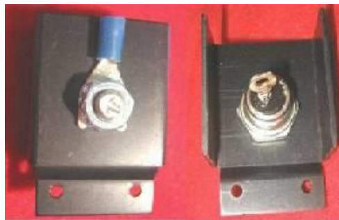
Figure 7. Power diode is connected to a heat sink.
