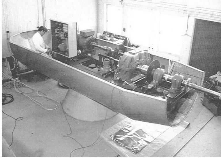
Figure 4. Nacelle interior of the Saab Scania wind turbine.
