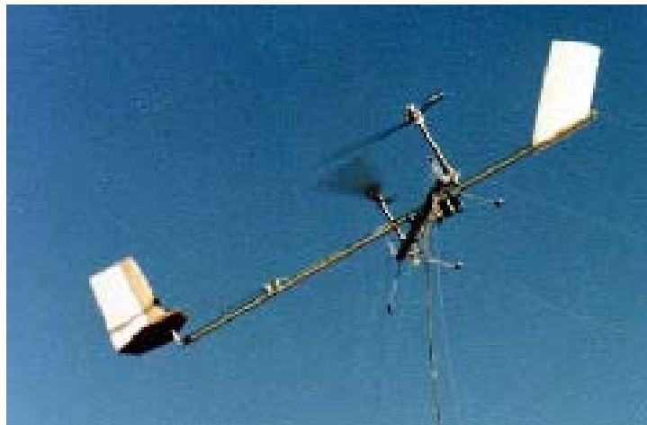
Fig. 12: Flying Electric Generator (FEG) with two contra rotating rotors.
