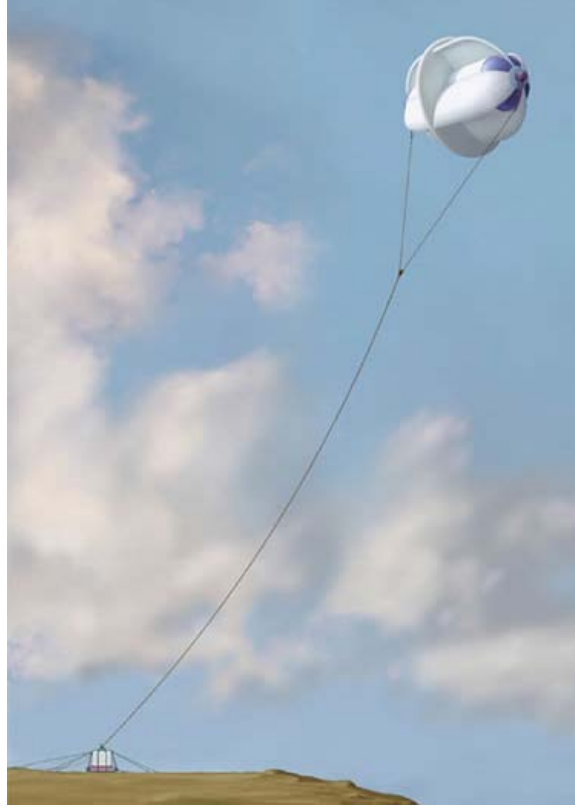
Fig. 2: Tethering of an air rotor system.
