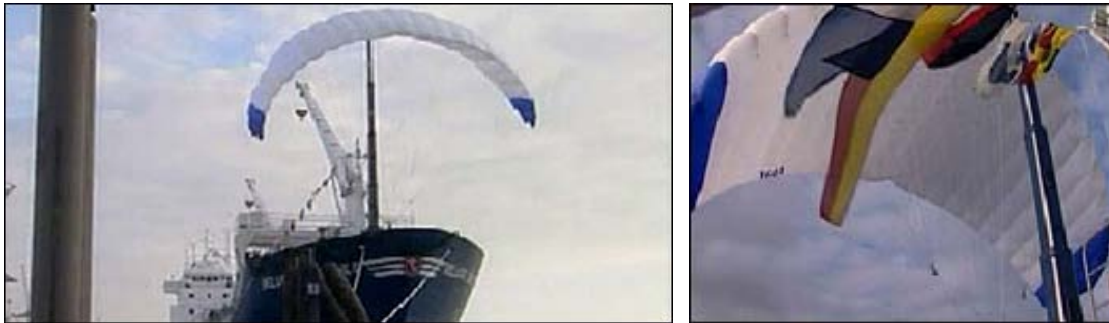
Fig. 1: Kite attached to a 15 meters high mast helps propel a German ship for a trip across the Atlantic. Source: BBC.
