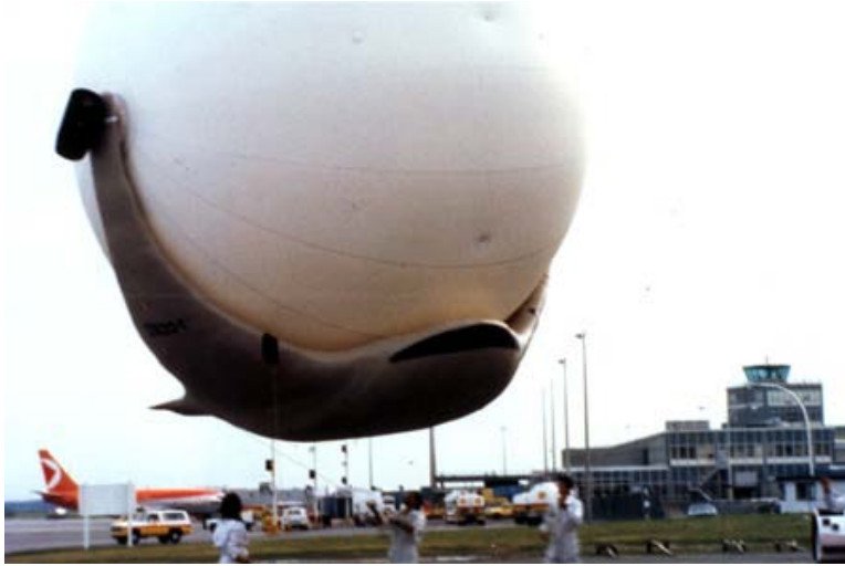
Fig. 4: Magnus Effect air-ship.
