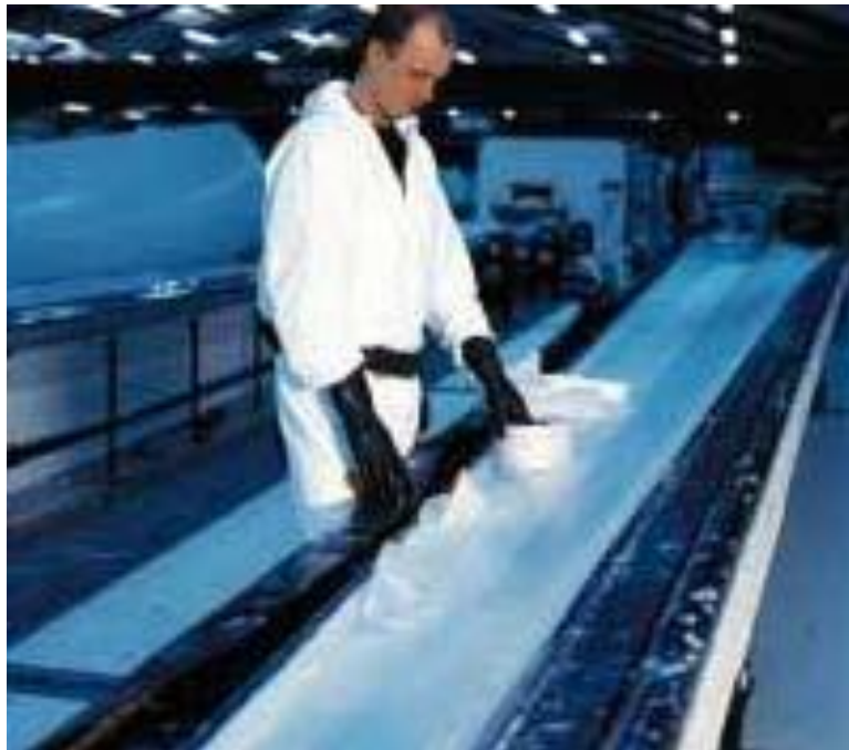
Figure 9. Wind rotor blade assembly.
