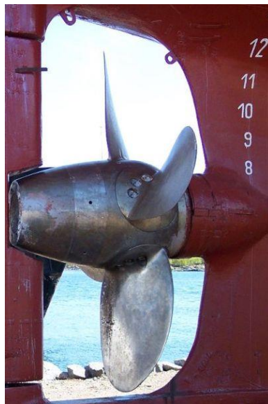
Figure 16. Ship variable pitch propeller blade design.
