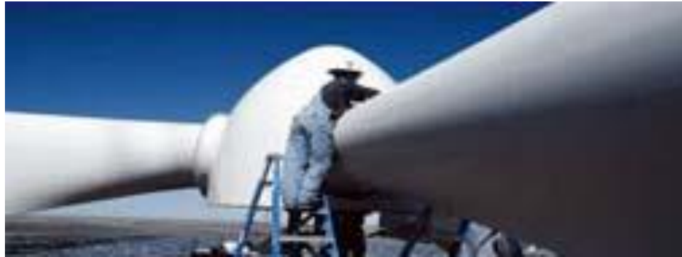
Figure 1. Rotor blade and hub showing its airfoil cross sectional shape.
