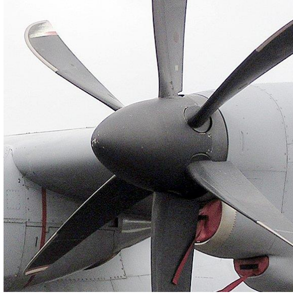
Figure 15. Lockheed Hercules C130J swept blade propeller design.
