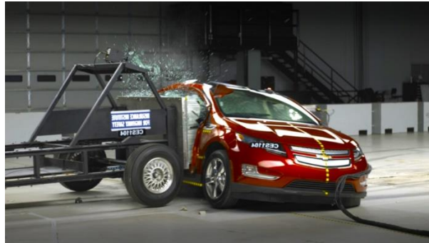
Figure 2. National Highway Traffic Safety Administration (NHTSA) testing of General Motors side impact safety of the Volt electric vehicle. Source: NHTSA.
