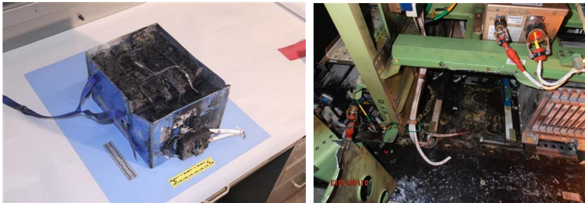
Figure 1. Spontaneously-occurring thermal damage in newly-introduced Li-ion batteries Auxiliary Power Unit (APU) battery in the Boeing 787 Dreamliner Japan Airlines airplane, January 7, 2012 at Logan Airport. Source: National Transportation Safety Board (NTSB).
