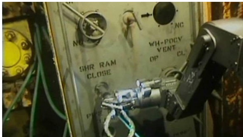
Figure 74. Underwater robot submarine attempted to activate the hydraulic shear rams on the Deepwater Horizon's blowout preventer on April 22, 2010 to close off the flow of oil from the Macondo well.
