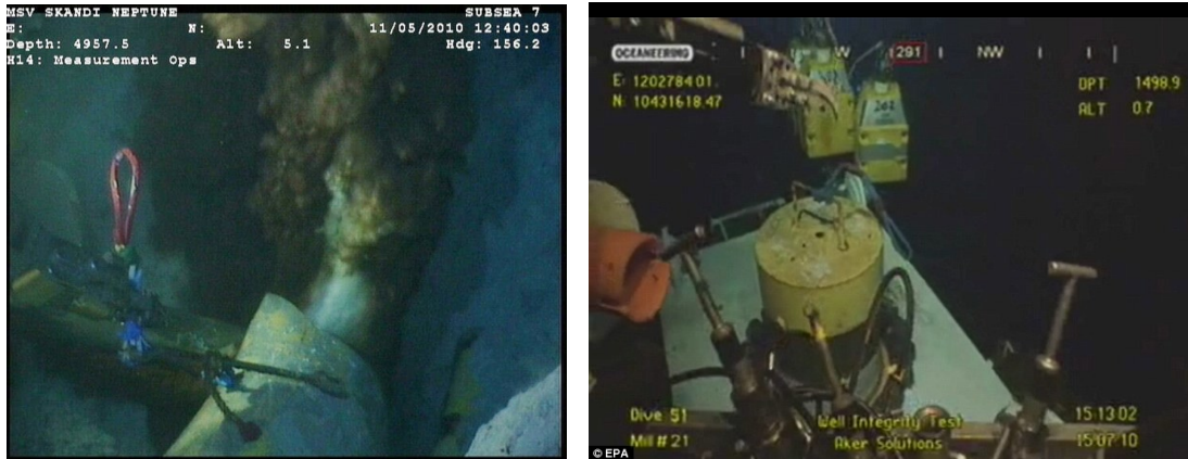
Figure 73. Leaking and capped underwater oil well.
