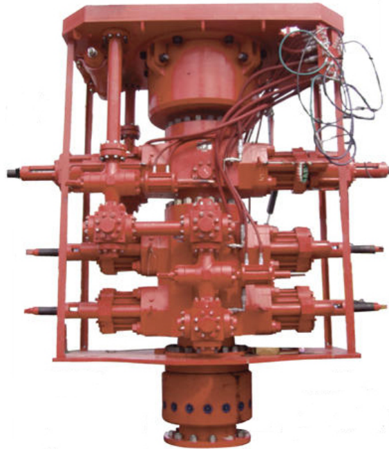
Figure 72. Blowout preventer, BOP is bolted to the top of the well on the sea floor. The hydraulic rams are horizontal piston-like protrusions. They are designed to cut and seal the pipe in an emergency, shutting off the flow of oil. Height: 50 ft or 15.2 m, weight: 500,000 lb or 226,000 kg.
