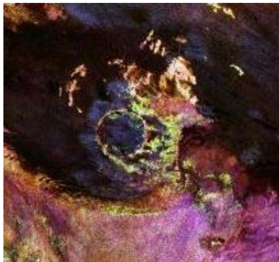
Figure 7. Gravity map of the 65 million years old buried Chicxulub 110-189 miles diameter crater in the Yucatan Peninsula, Mexico. It is thought to have trapped marine sediment eventually forming the giant Cantarell oil deposit. White dots are cenotes, (from Maya dz'onot), are natural wells or reservoirs, common in the Yucatán Peninsula, formed when a limestone surface collapses, exposing water underneath. The major source of water in the modern and ancient Yucatán, they are also associated with the cult of the rain gods, or Chacs. Source: USGS.
