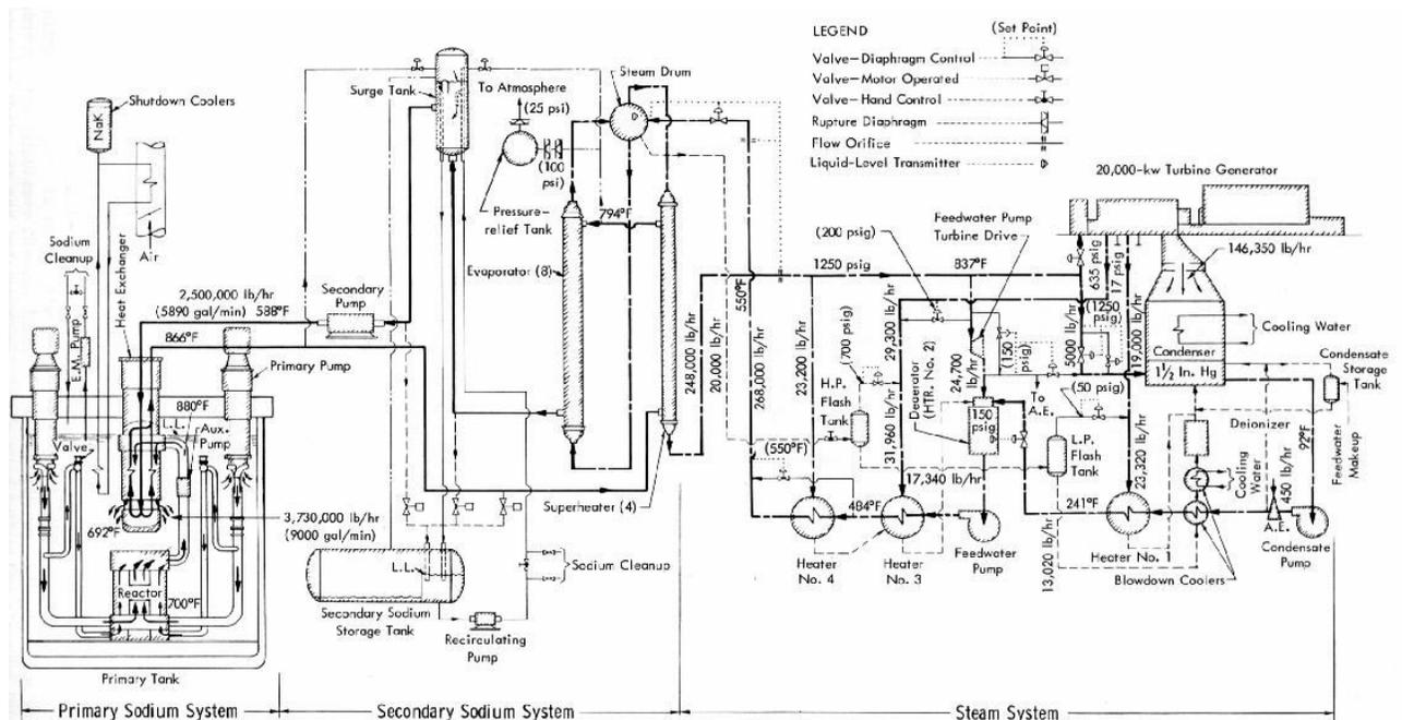
Figure 1. Experimental Breeder Reactor , EBR-II flow chart showing intermediate sodium cooling circuit.
