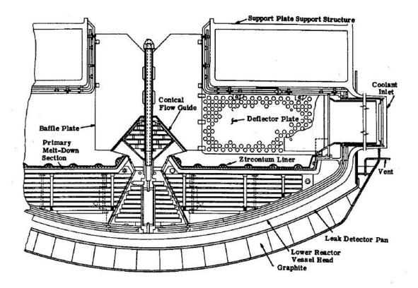
Figure 4. Fermi-1 core coolant inlet, dispersion and meltdown section. The loosened plates Zircaloy at the inlet coolant flow were broken loose to partially or totally obstruct one or the other fuel subassemblies inlet plenums during startups and shutdowns.
