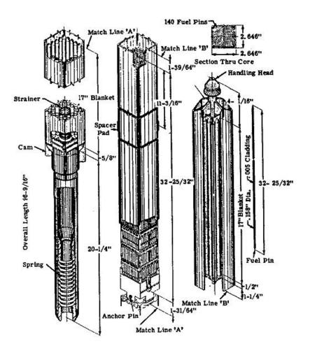
Figure 3. Fuel subassembly in the Fermi-1 reactor.
