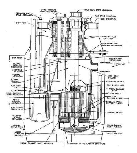
Figure 2. Fermi 1 vessel elevation.
