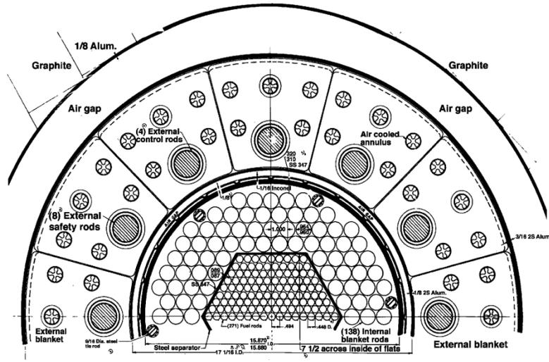
Figure 2: Experimental Breeder Reactor 1, EBR-1 core configuration.
