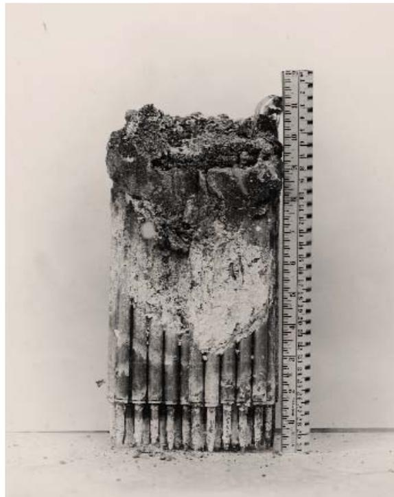
Figure 3. Damaged core of EBR-1 reactor from 1955 core meltdown.
