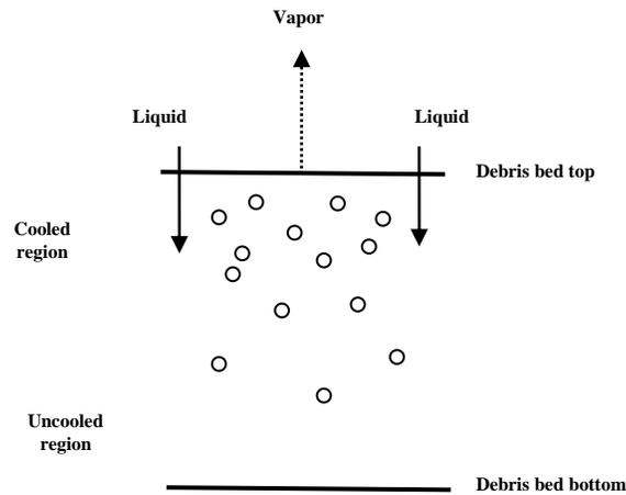
Figure 3. Closed bed debris bed cooling.
