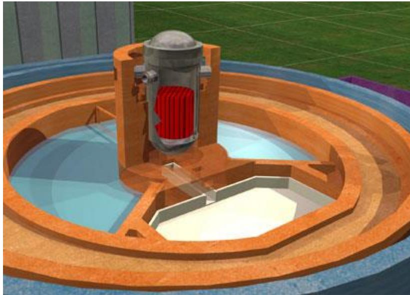
Figure 5. Corium and debris bed cooling system in the Evolutionary PWR, EPWR.
