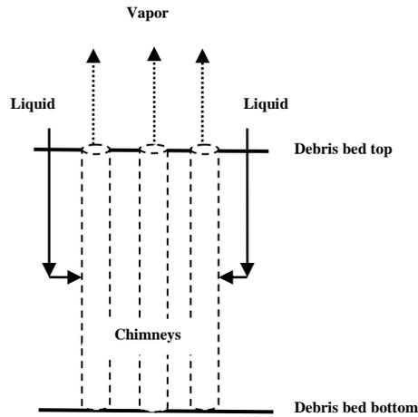
Figure 2. Debris bed chimneys cooling.
