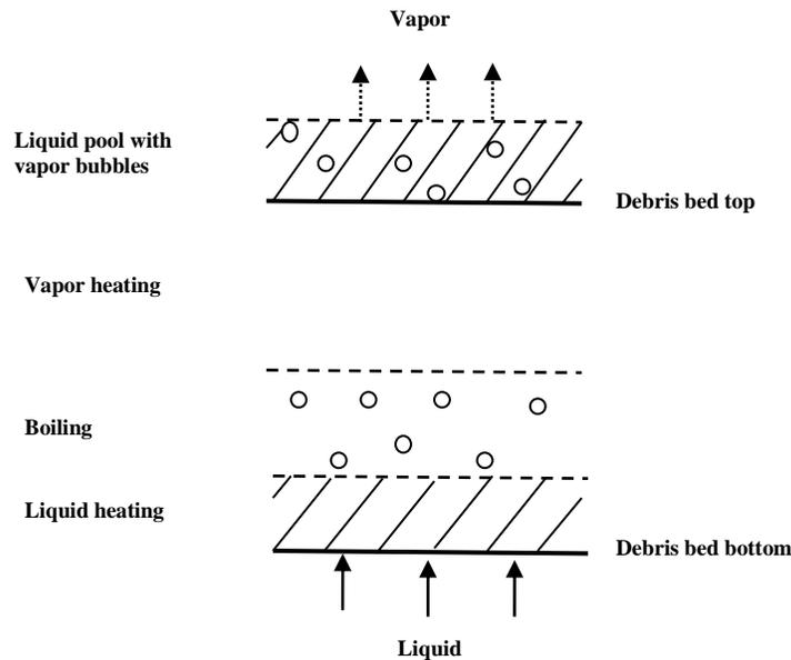
Figure 4. Multilayered once-through debris bed cooling.
