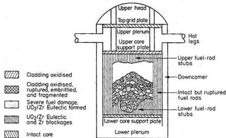
Figure 1. Debris bed resulting from the core damage in the Three Miles Island accident.
