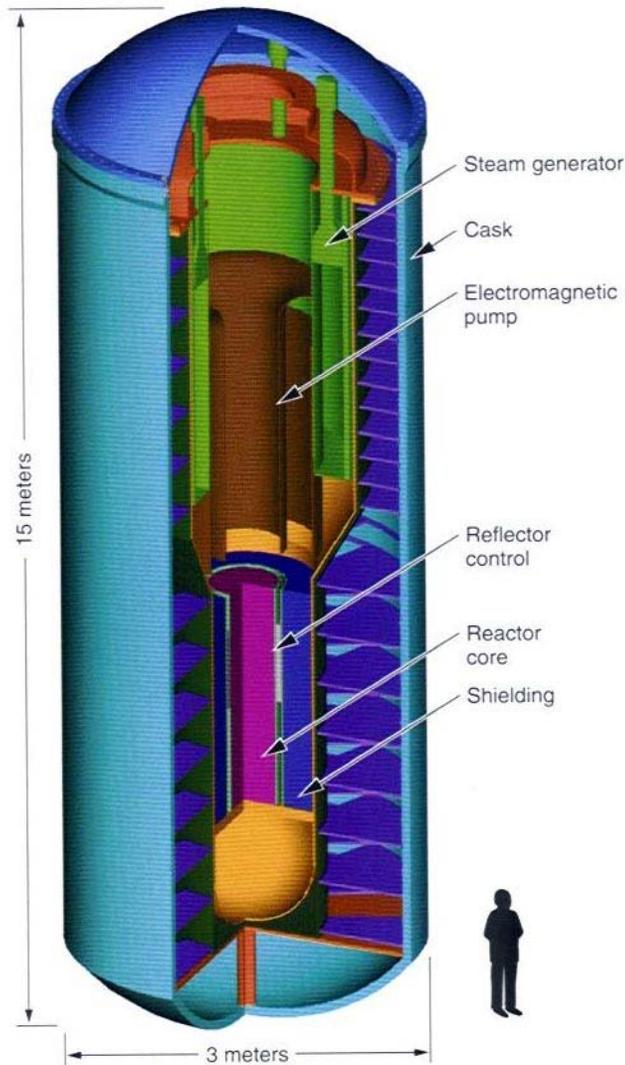
**Fig. 4: Schematic of Small, Sealed, Transportable, Autonomous Reactor, SSTR.**
