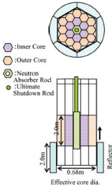
**Fig. 2: Core design of the 4S reactor concept.**
