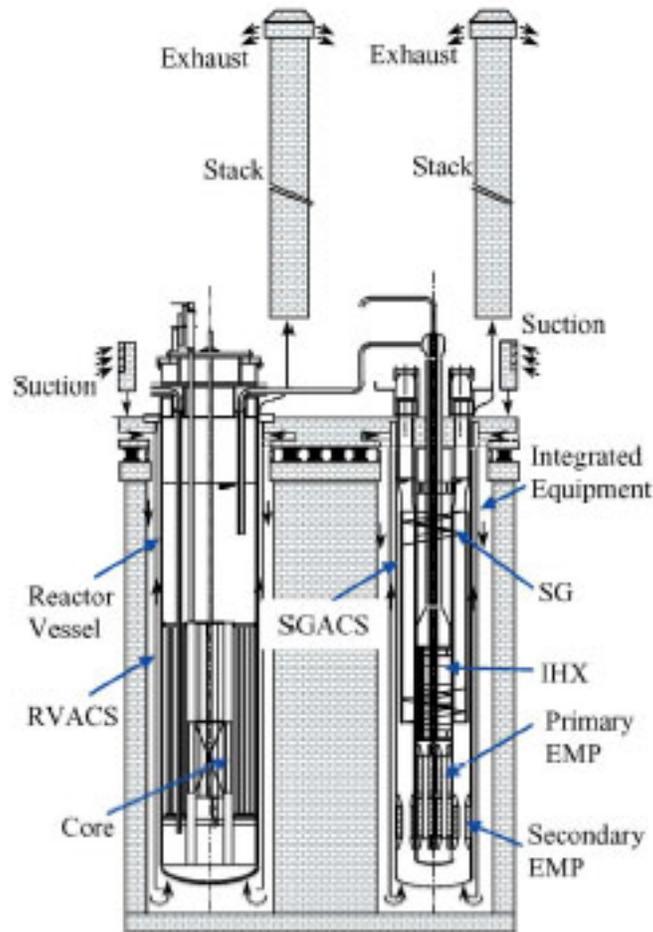
**Fig. 3: Parallel configuration of the 4S reactor showing its core and Intermediate Heat Exchanger (IHX).**
