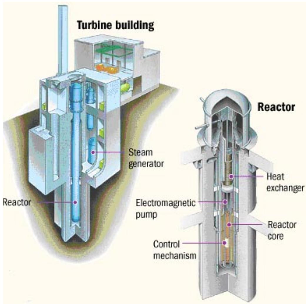
**Fig. 1: 4S Toshiba reactor configuration.**
