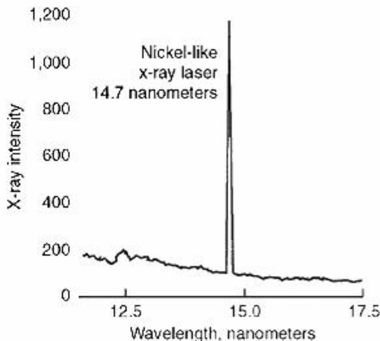
**Fig. 4: Nickel like x ray laser lasing at 14.7 nanometer with a line brighter than the other emission lines.**
