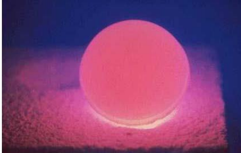
Figure 4. Plutonium 238 disc that glows red-hot from its internal heat generation.
