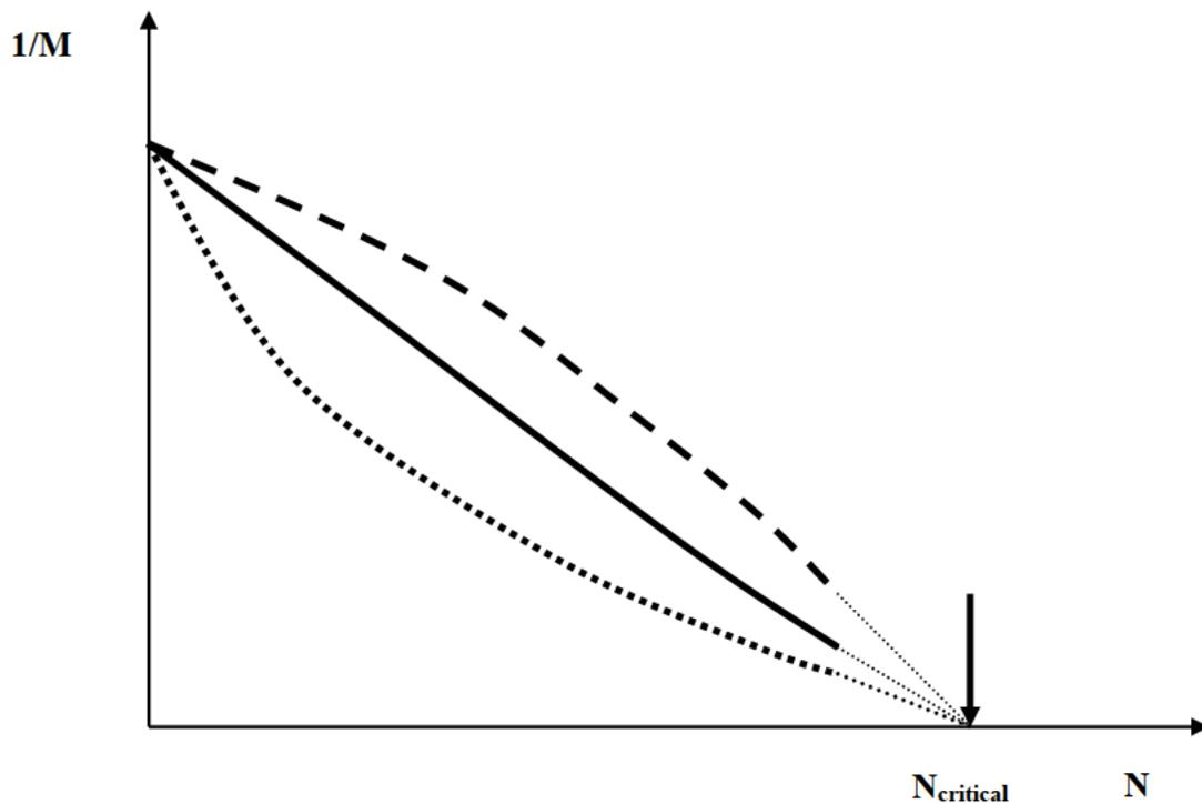
Figure 6. Reciprocal counting rate from several detectors is used with an external source to determine the critical number of fuel assemblies during reactor startup.
