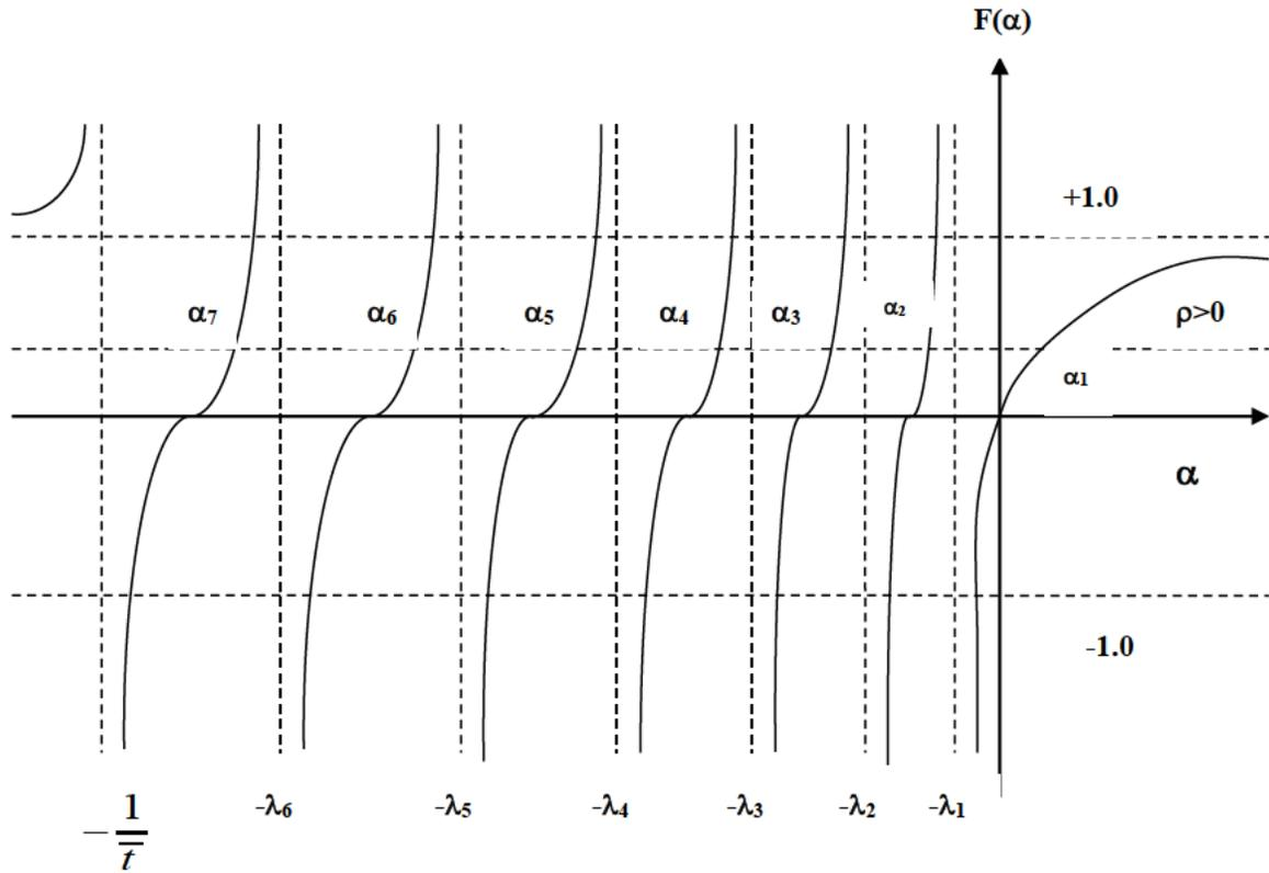
Figure 2. Characteristic function  $F(\alpha)$  for 6 groups of delayed neutrons.
