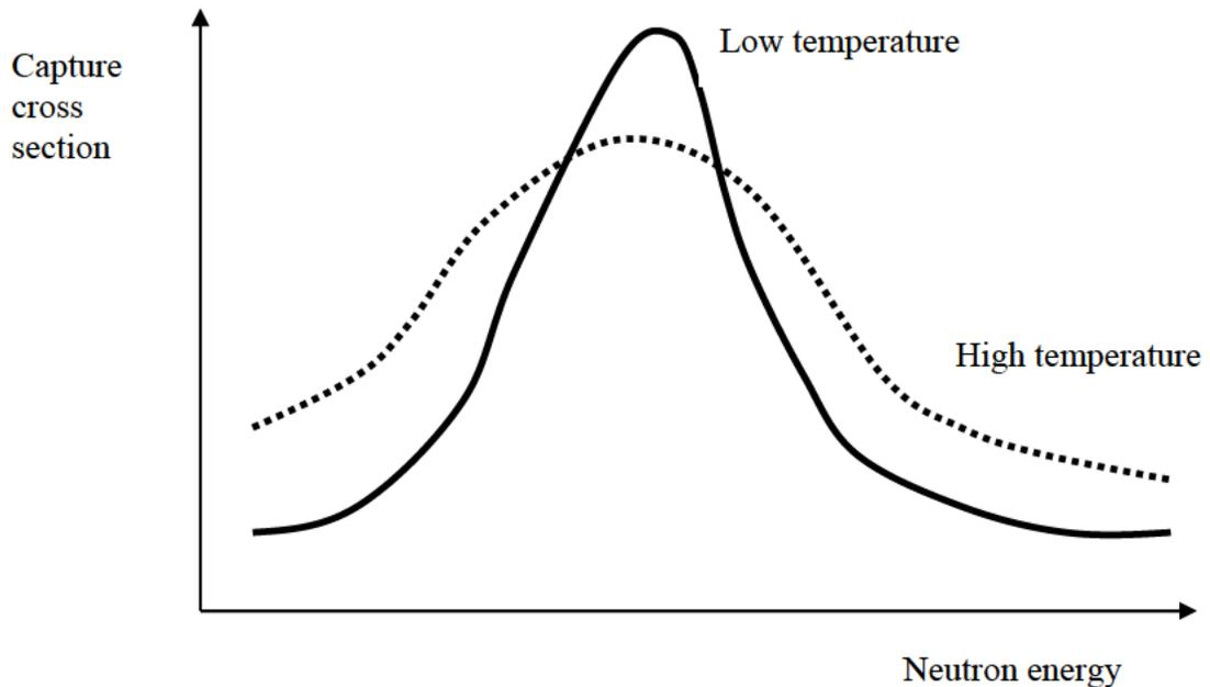
Figure 4. The nuclear Doppler Effect involves a widening of the neutron absorption cross sections resonances with an increase in temperature.
