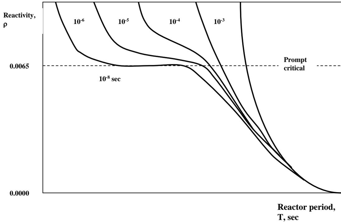
Figure 3. Reactor reactivity and period for different neutron generation times.
