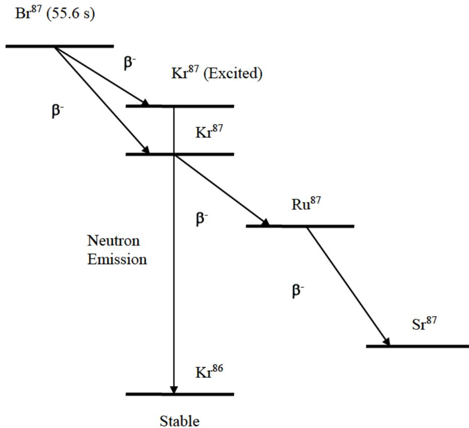
Figure 1. Delayed neutron emission from Bromine<sup>87</sup>.
