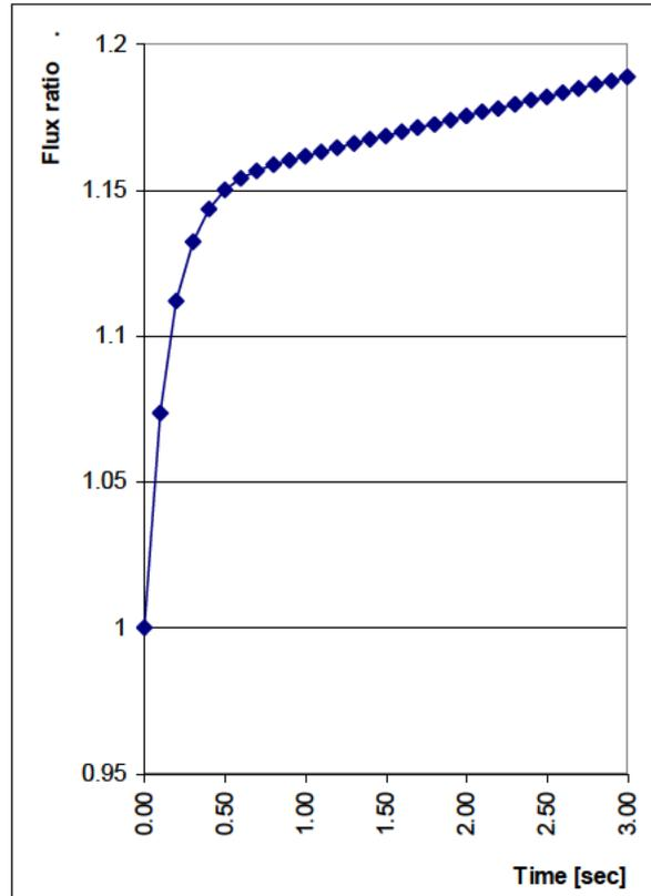
Figure 5. During the first few seconds the flux ratio increases and at about half a second it rises according to the stable reactor period.
