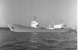
Figure 9. The NS Otto Hahn nuclear bulk carrier.
