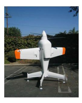
Figure 93. Skytote counter rotating vertical-landing UAV. Source: AeroVironment.
