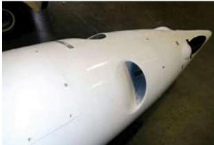
Figure 121. Dual propellers and distributed multi jets propulsor inlets (right) and outlets (left).
