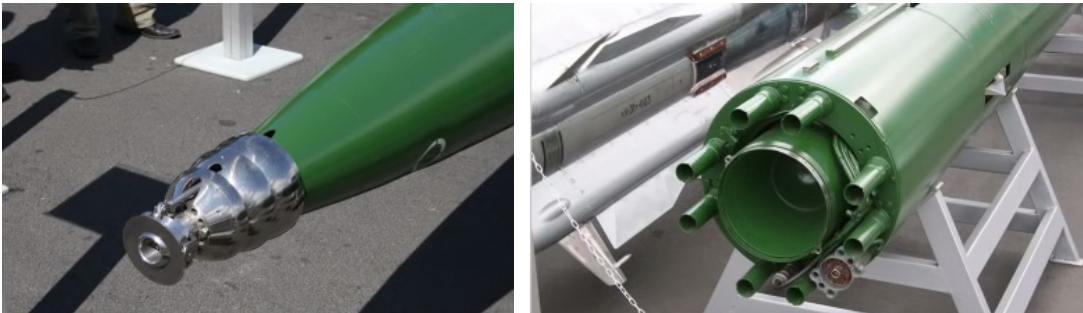
Figure 143. Super-cavitation under-water vehicles are alleged to be capable of reaching 230 mph speeds.
