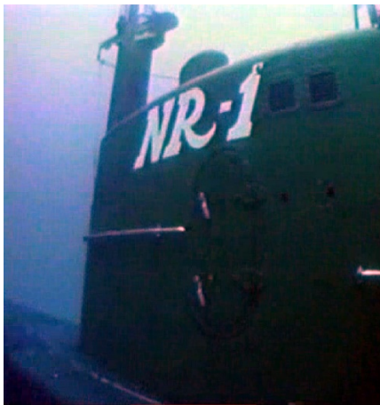
Figure 58. The NR-1 deep submergence submarine and its mother ship the SSV Carolyn Chouest. It could dive to three times the depth of other submarines, and was equipped with wheels to move on the ocean floor and a robotic arm. It has been replaced with remotely controlled submersibles.
