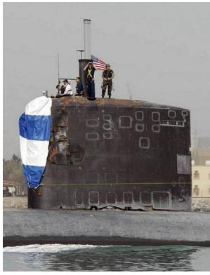
Figure 77. The collision of the Hartford with the New Orleans on March 20, 2009 caused damage to its communication gear and bent its sail.
