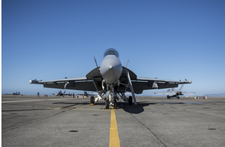
Figure 137. Boeing EA-18G Growler electronic jamming warfare aircraft carries pods at tips of wings.
