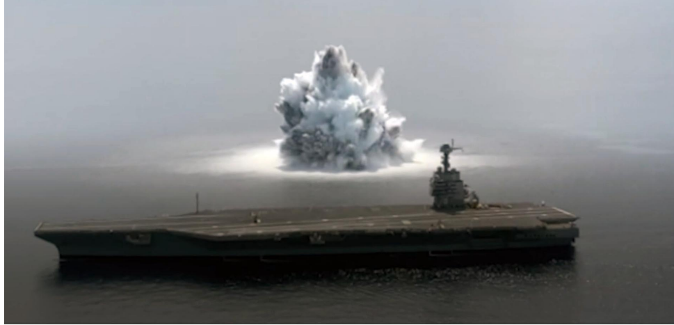
Figure 43. CVN-78 Gerald R. Ford features. The $17.5 billion carrier Gerald R. Ford uses for the first time an Electromagnetic Aircraft Launch System, or EMALS system, which replaces traditional steam-based carrier aircraft launch systems. “Full Ship Shock Trial” under battle conditions using a 40,000 lbs explosive charge. Source: USA Navy
