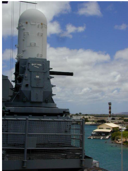
Figure 38. The Phalanx radar-guided gun, nicknamed as R2-D2 from the Star-Wars movies, is used for close-in ship defense. The radar controlled Gatling gun turret shooting tungsten armor-piercing, explosive, or possibly depleted uranium munitions on the USS Missouri, Pearl Harbor, Hawaii. Photo: M. Ragheb.
