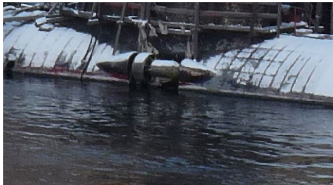
Figure 61. Multipurpose nuclear deep station AS 13 pr. 1910. The right front thruster in retracted position without cover.
