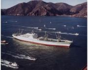
Figure 8. The Savannah, the first nuclear USA merchant ship used Low Enriched Uranium (LEU) fuel in the range of 4.2-4.6 percent. It was powered by a single 74 MW Babcock and Wilcox nuclear core powering two De Laval steam turbines.
