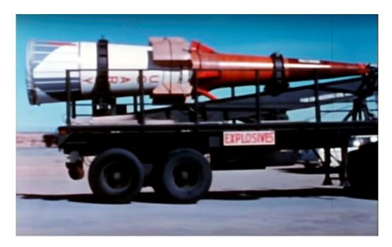
Figure 146. Sprint two-stage Surface to Air Missile SAM interceptor.
