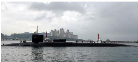
Figure 51. The USS Michigan carries 154 Tomahawk cruise missiles that can travel at 550 mph and a 60 special-forces unit with a SEAL combat insertion unit.
