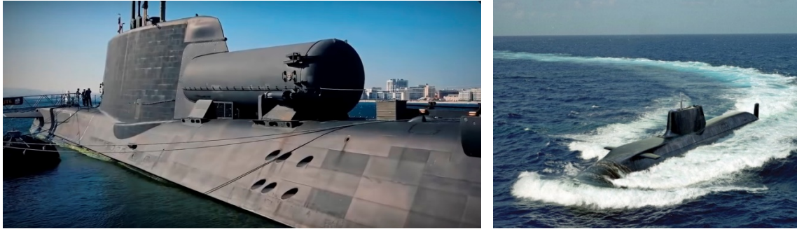
Figure 123. HMS Astute 48 class of attack submarine on rollout showing the lampshade noise suppression duct surrounding its shrouded jet propulsor. Source: BAE Systems, UK.
