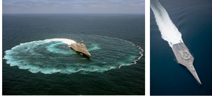
Figure 95. LCS 2 Independence-class Littoral Combat Ship high maneuverability. The generated wake from a sharp turn can sink small fast attacking craft.
