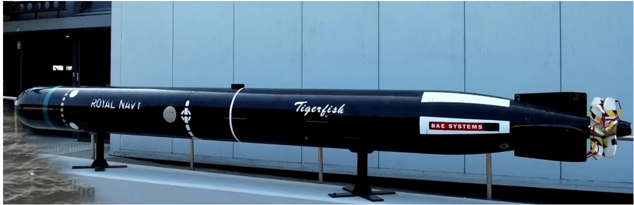
Figure 142. Mark 24 Tigerfish electric torpedo replacing compressed air torpedoes.
