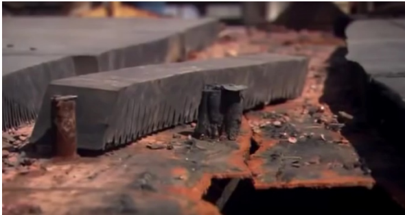
Figure 103. Installation of skin surface “anechoic” rubber or urethane tiling to absorb sonar signals on outer surface of hull of a UK nuclear submarine that lost some tiles (top). Peeling urethane tile on Virginia class vessel, USA. Russian Akula class of submarines acoustic coating (bottom).
