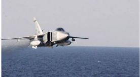
Figure 135. Russian Sukhoy-24 buzzing USS Donald Cook destroyer. The jamming was possibly produced by the two pods; other than the fuel tanks, visible under the wings of the aircraft. On larger aircraft, more massive versions seem to be positioned at the tips of the wings. Source: USA Navy.
