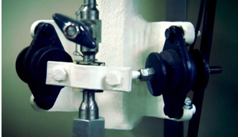
Figure 102. Rubber shock absorbers for vibration suppression.
