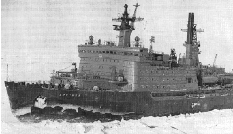
Figure 67. Nuclear icebreaker Arktika used Intermediate Enriched Uranium (IEU) of 30-40 percent as fuel.
