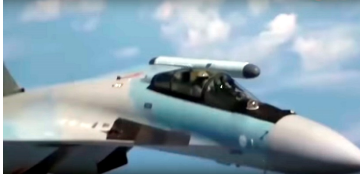
Figure 136. Pods of Khibiny electronic warfare system mounted on Russian aircraft.
