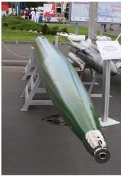
Figure 144. VA 111 Shkval Russian super-cavitation torpedo's nozzle is controlled by a four-wire system at the nose.
