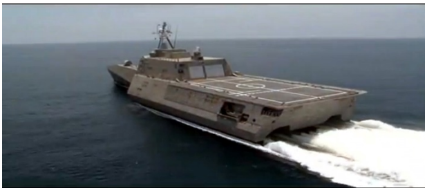
Figure 94. Trimaran Littoral Combat Ship uses water jets propulsion for Independence-class stealth ships. Source: Austal, USA Navy.
