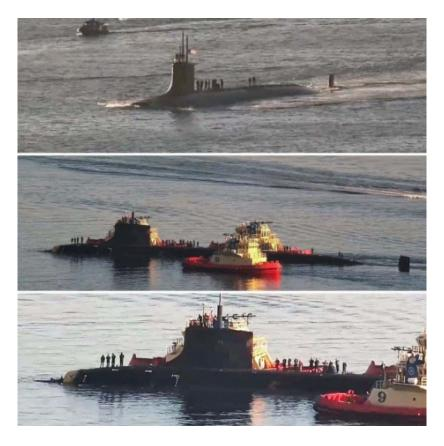
Figure 81. The bow of the nuclear submarine "USS Connecticut" SSN 22 Sea-Wolf Class was crumpled almost to the wheelhouse. Damage to the sub's sonar dome left it unable to travel underwater.
