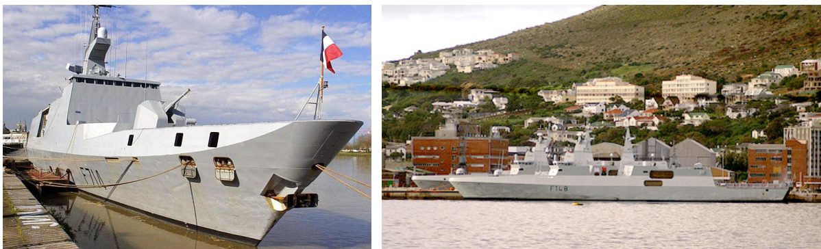
Figure 82. Stealth radar deflecting technology implemented into a French Lafayette class frigate, 2001 (left). The South African stealth Valour class frigates, built by Blohm + Voss from Hamburg, Germany to the MEKO A-200SAN design, uses both screws and water jets, in a “Waterjet and Refined Propeller” or WARP arrangement, with three shaft lines. A single GE
