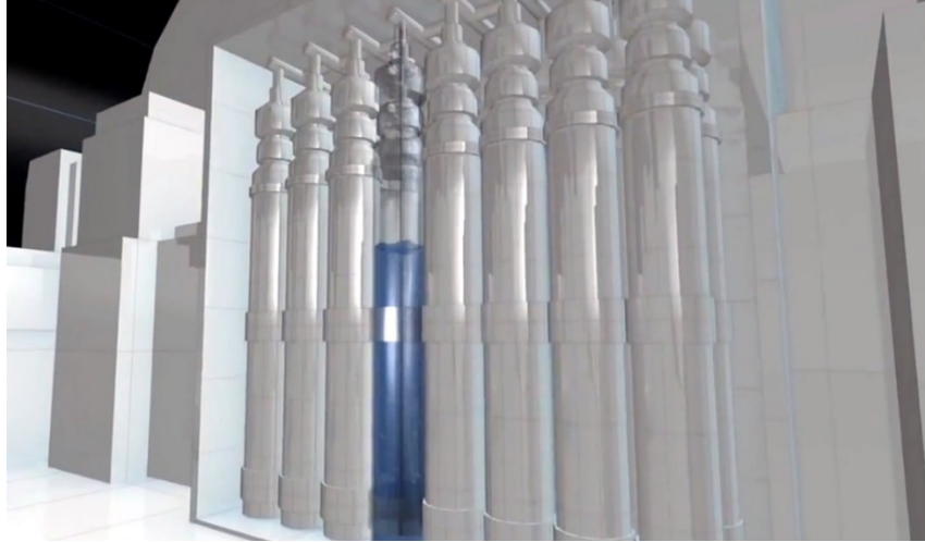
Figure 104. Schematic of water electrolysis system for generation of breathing oxygen. The oxygen and hydrogen could be stored for silent operation using fuel cells to drive electrical motors.
