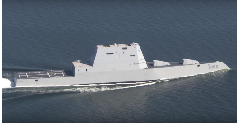
Figure 134. Zumwalt class destroyer all-electric naval vessel. Source: USA Navy.
