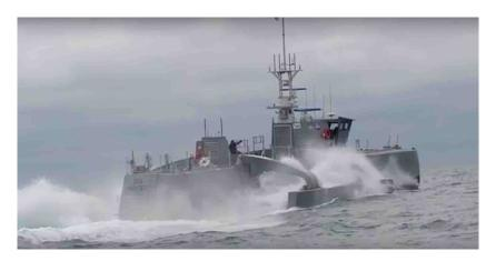
Figure 119. Sea hunter drone single-float catamaran for Anti-Submarine Warfare (ASW).
