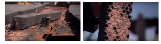
Figure 103. Installation of skin surface "anechoic" rubber or urethane tiling to absorb sonar signals on outer surface of hull of a UK nuclear submarine that lost some tiles (top). Peeling urethane tile on Virginia class vessel, USA. Russian Akula class of submarines acoustic coating (bottom).
