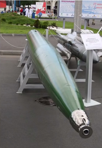
Figure 144. VA 111 Shkval Russian super-cavitation torpedo's nozzle is controlled by a four-wire system at the nose.
