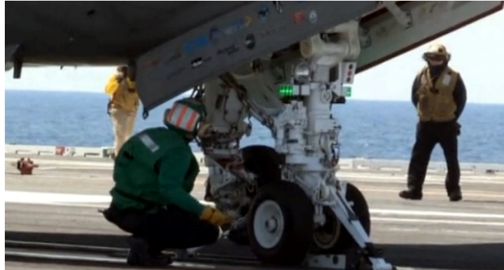
Figure 90. Northrup- Grumman X47 steam catapult. Source: USA Navy.
