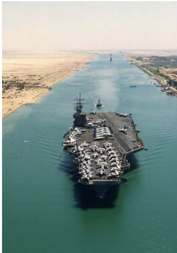
Figure 1. Nuclear aircraft carrier USS Theodore Roosevelt, Nimitz Class CVN-71, powered with two A4W (A for Aircraft carrier, 4 for fourth generation and W for Westinghouse) nuclear reactors with 100 MW of rated power each, crossing the Suez Canal, Egypt, during the first Gulf War, January 1991. Source: USA Navy.
