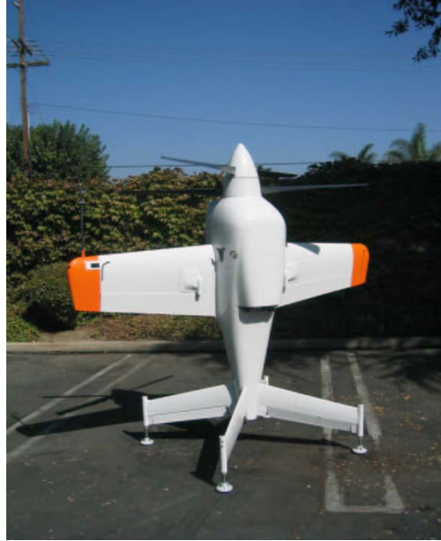
Figure 93. Skytote counter rotating vertical-landing UAV. Source: AeroVironment.
