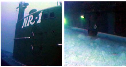
Figure 58. The NR-1 deep submergence submarine and its mother ship the SSV Carolyn Chouest. It could dive to three times the depth of other submarines, and was equipped with wheels to move on the ocean floor and a robotic arm. It has been replaced with remotely controlled submersibles.
