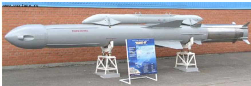
Figure 49. Yakhont P800 Russian cruise missile, 138 miles range. Source: Ruaviation.
