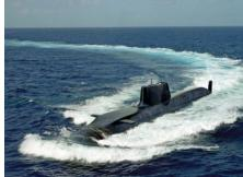
Figure 123. HMS Astute 48 class of attack submarine on rollout showing the lampshade noise suppression duct surrounding its shrouded jet propulsor. Source: BAE Systems, UK.
