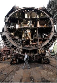
Figure 108. Double-hulled Russian submarine cross-section with missile tubes positioned in annular space.
