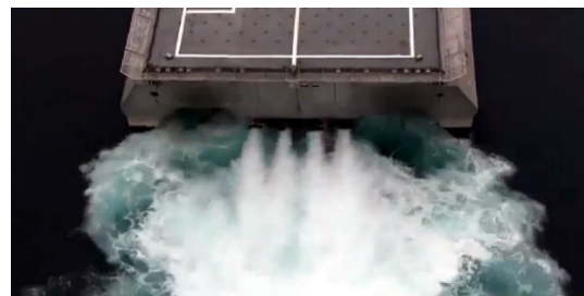
Figure 94. Trimaran Littoral Combat Ship uses water jets propulsion for Independence-class stealth ships. Source: Austal, USA Navy.
