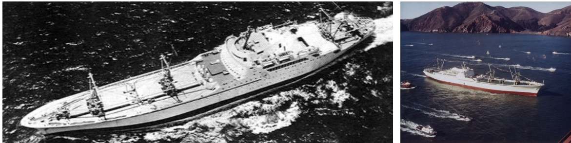
Figure 8. The Savannah, the first nuclear USA merchant ship used Low Enriched Uranium (LEU) fuel in the range of 4.2-4.6 percent. It was powered by a single 74 MW Babcock and Wilcox nuclear core powering two De Laval steam turbines.
