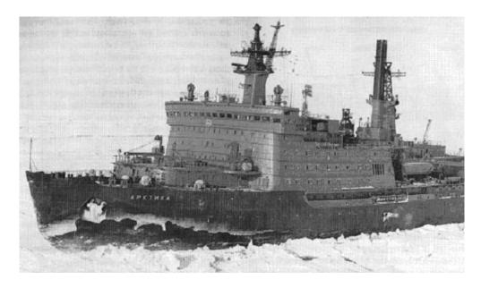
Figure 67. Nuclear icebreaker Arktika used Intermediate Enriched Uranium (IEU) of 30-40 percent as fuel.
