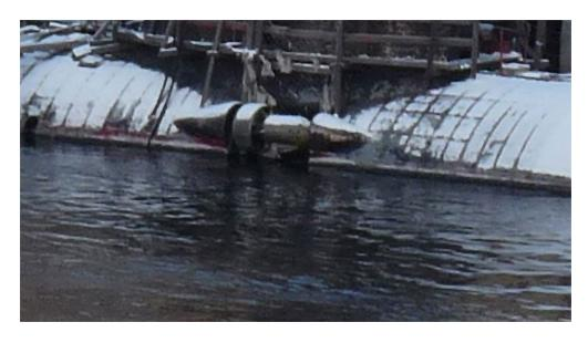
Figure 61. Multipurpose nuclear deep station AS 13 project 1910. The right front thruster in retracted position without cover.
