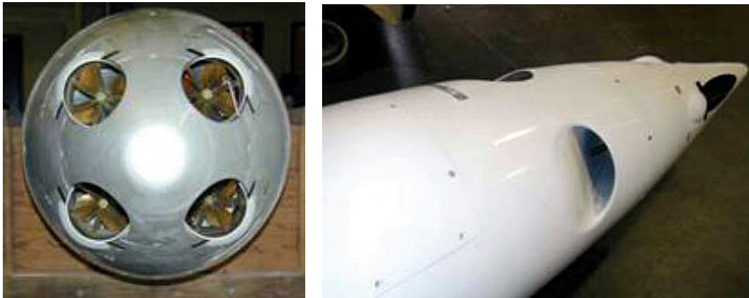
Figure 121. Dual propellers and distributed multi jets propulsor inlets (right) and outlets (left).
