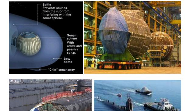
Figure 72. Location of sonar dome on the Astute class of submarines, UK. USS San Francisco SSN 711 accident, January 8, 2005. Damage from the glancing collision to the bow dome and to the double hull structure can be observed. A bulge over the hull can also be noticed.
