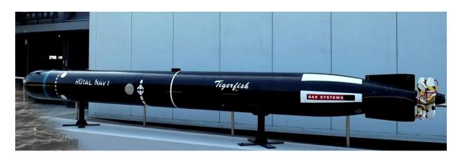
Figure 142. Mark 24 Tigerfish electric torpedo replacing compressed air torpedoes.
