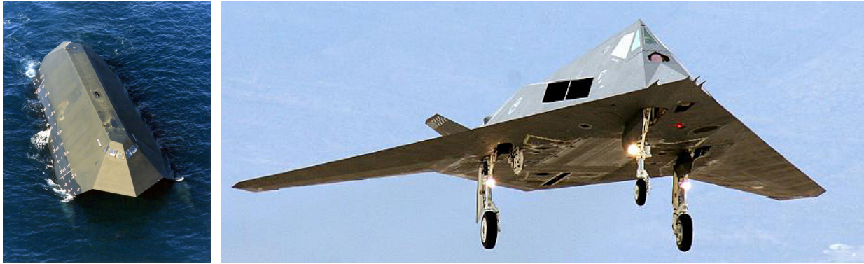
Figure 80. The Sea Shadow stealth ship in 1990 and in 2004 used radar deflecting technology used in the F-117 Nighthawk stealth fighter. Source: USAF.
