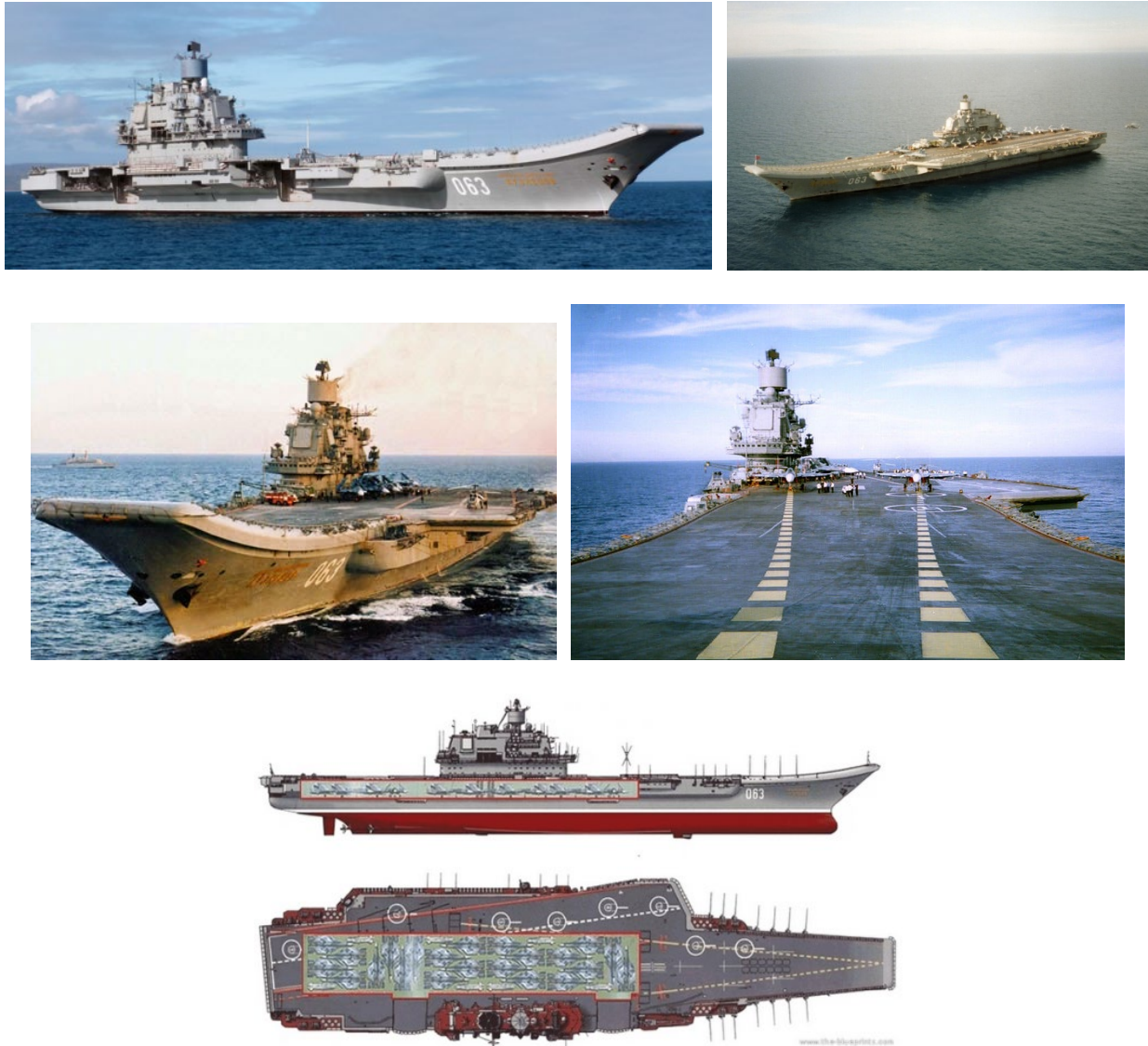
Figure 27. Admiral Kuznetsov Russian non-nuclear aircraft carrier. Uses 8 conventional steam boilers. Because aircraft carriers are banned from passing through the Bosphorus straits under the 1936 Montreux Convention, and otherwise it could not enter the Black Sea, it is referred to as a "battle-cruiser."
